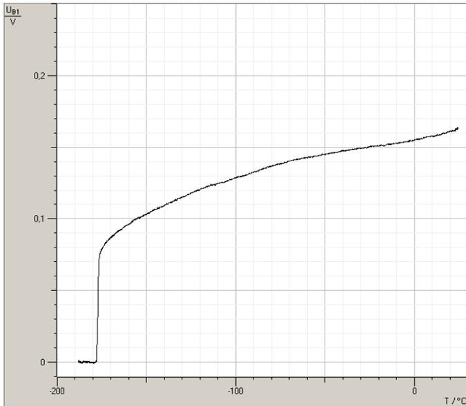
Fig. 4: Voltage drop at the transition temperature of approximately  $-180\text{ }^{\circ}\text{C}$ .
