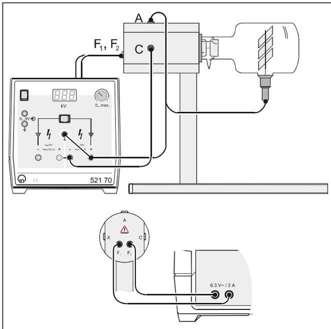
Fig. 1: Setup for observing cathodoluminescence
