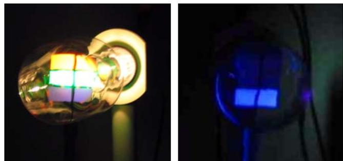
Fig. 3: Cathodoluminescence (left) and photoluminescence (right)
