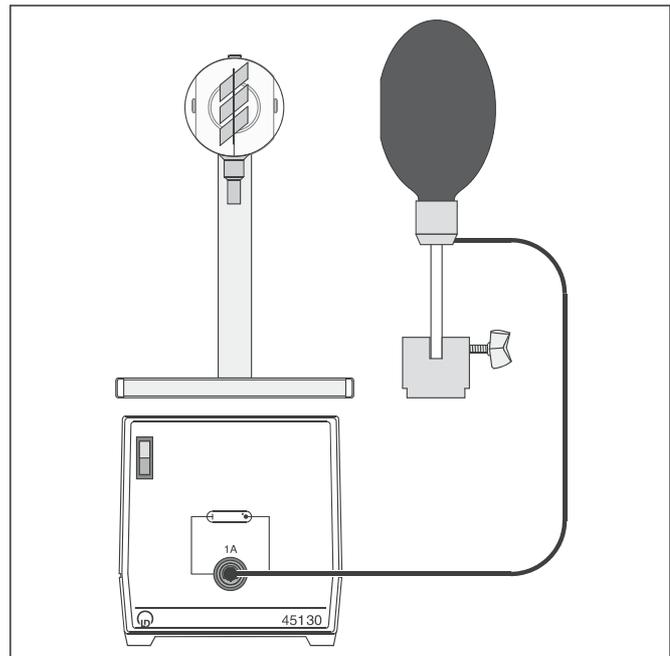
Fig. 2: Setup for observing photoluminescence
