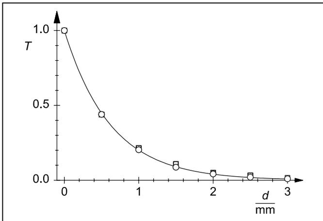
Fig. 2 Transmittance  $T$  as a function of the thickness  $d$  of the aluminum absorbers
