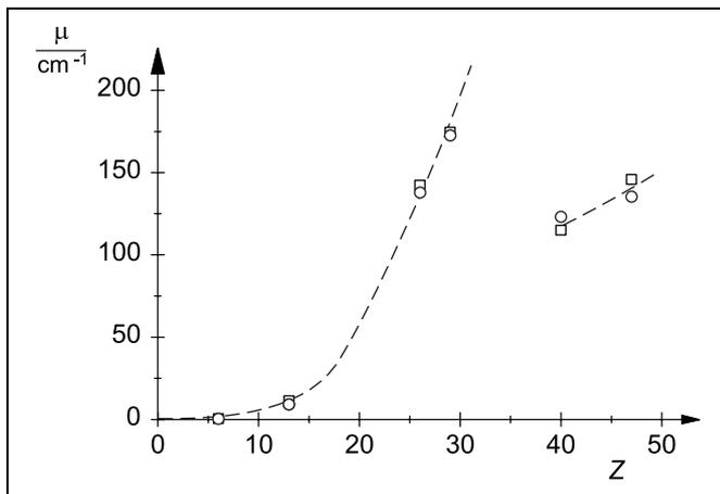
Fig. 4 Linear attenuation coefficient  $\mu$  as a function of the atomic number  $Z$  of the absorber
