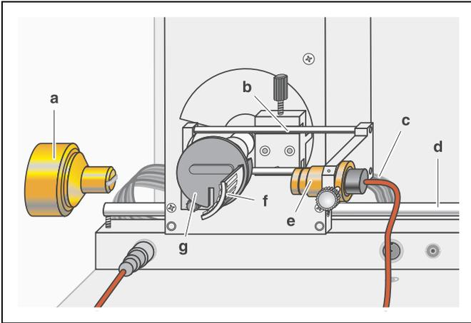
Fig. 1 Setup for investigating the attenuation of x-rays as a function of the thickness of the absorber material.
