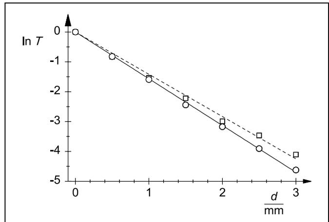
Fig. 3 Floating-point representation of transmission  $T$  as a function of the thickness  $d$  of the aluminum absorbers
