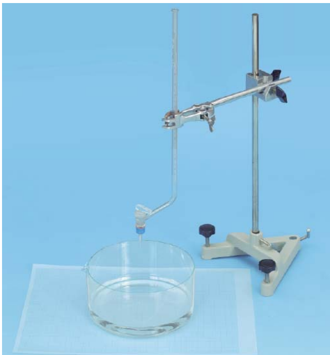
Fig. 1: Experimental setup to estimate the size of oil molecules.
