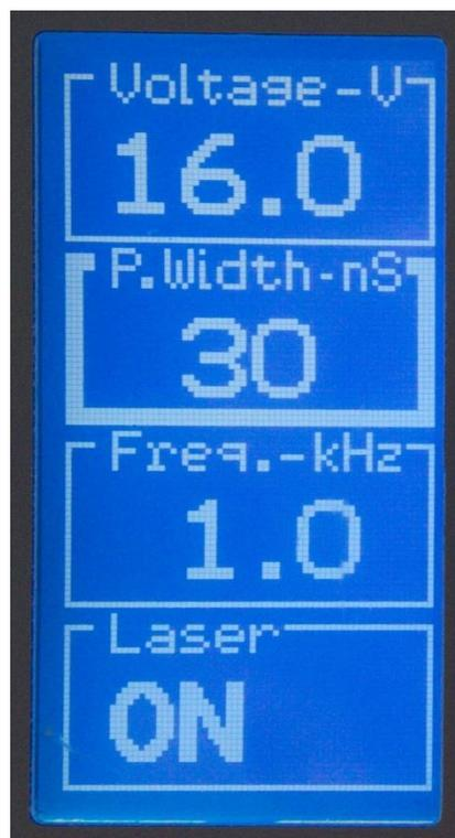
To set the three values, turn the knob until the value to be set is highlighted by a thick white frame (Pulse Width in the image above), press the button for a few seconds, now the value starts to blink. Turning the knob changes the value immediately and another long press of the knob leaves the value setting and changes to the selection of the white frame.
