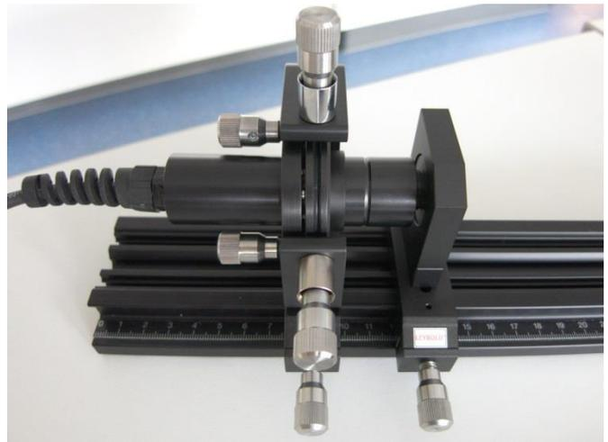
The receiver is built from the detector 474 331 held by a 474 209 together with a biconcave lens 474 104. Connect the BNC output to the second channel of the oscilloscope. The battery box contains a 9V block battery and a switch. Switch on the detector and put the lens a few cm in front of the detector.
