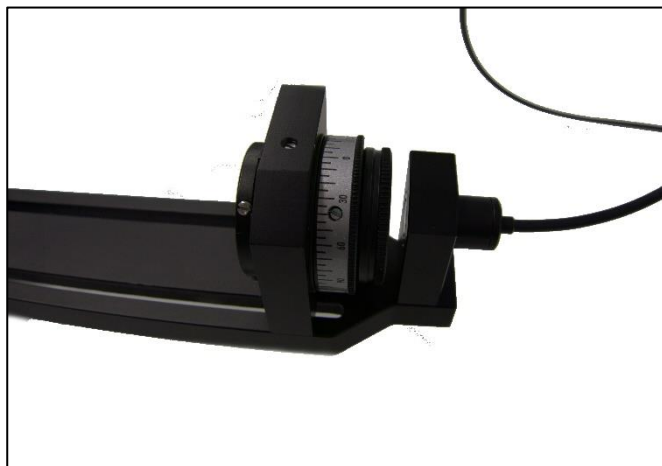
Fig. 15: Polarization filter in front of the photodetector.
