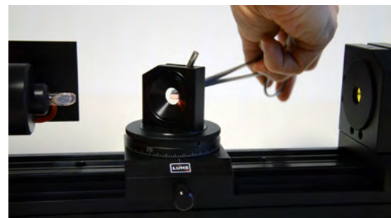
Fig. 47: Cleaning the BFT plate from both sides with a special formed cleaning pad
