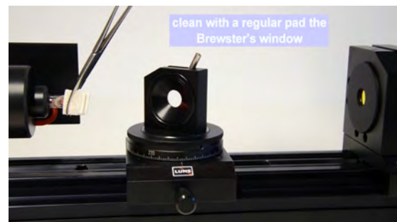
Fig. 46: Cleaning the Brewster window of the laser tube
