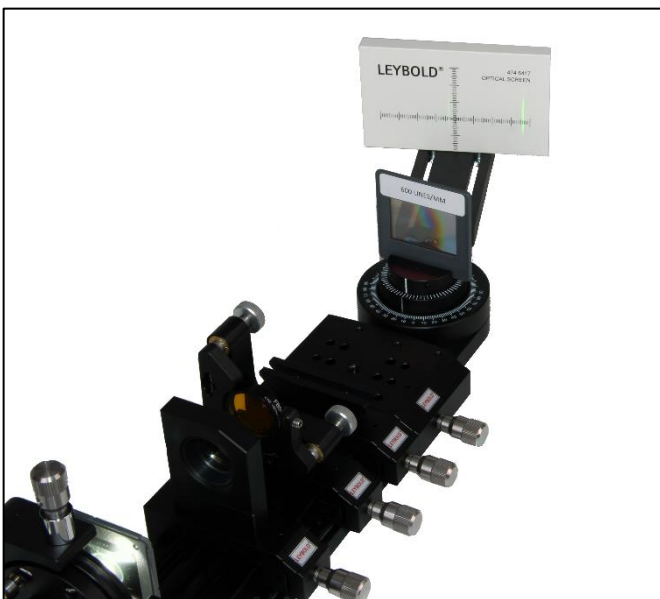
Fig. 8: Setup with interference filter 550 nm in adjustment holder 1 inch.
