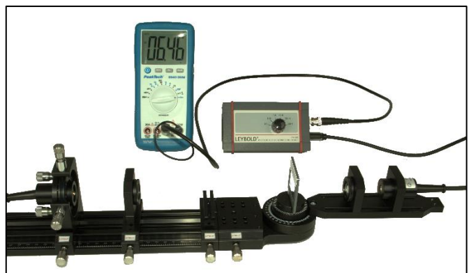
Fig. 9: Setup to measure the intensities using a NIR Lamp Setup on Bench:
