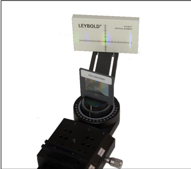
Fig. 7: Turning the swivel unit so that the y axis is in the middle of a coloured line.
