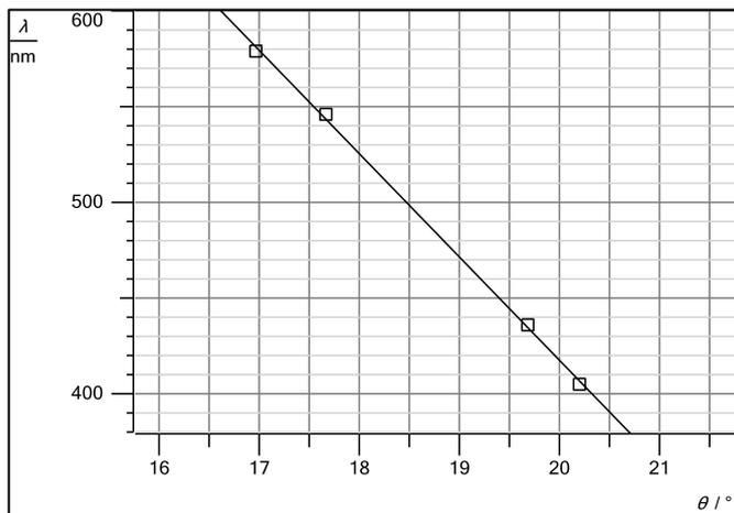
Fig. 13: Calibration fit of the 600 lines / mm grating.
