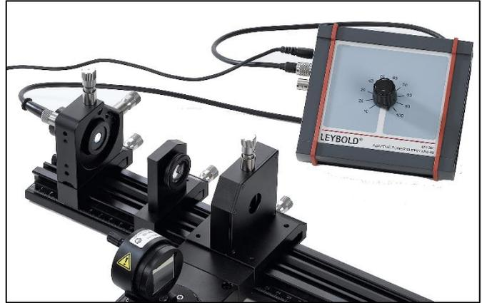
Fig. 8: LED Lamp and lens  $f = 40$  mm placed before the first slit.
