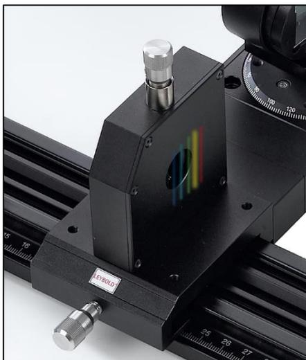
Fig. 10: Image of the first slit at the entrance of the second slit.
