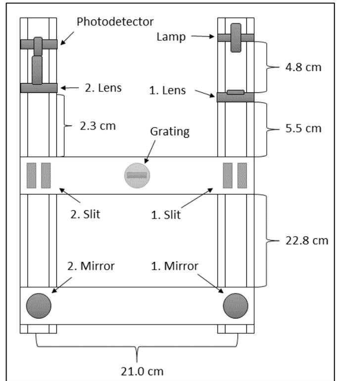
Fig. 11: Setup with distances of the elements.
