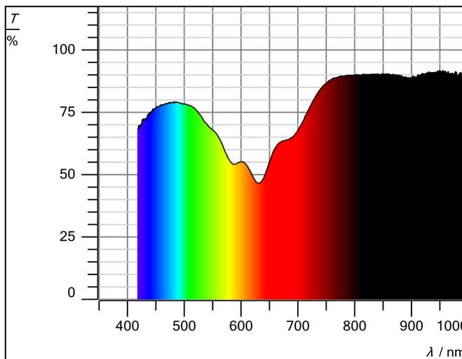
Fig. 19: Transmittance of the acrylic absorption filter.
