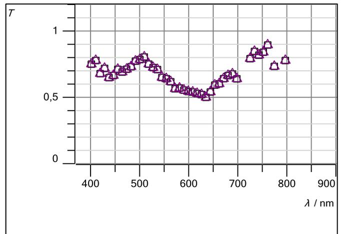
Fig. 18: Measured transmittance of the acrylic absorption filter.
