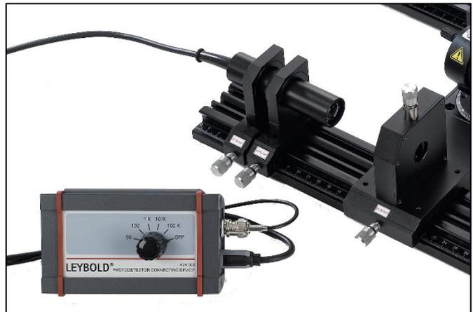
Fig. 9: Photodetector and Biconvex Lens  $f = 20$  mm behind the second slit.
