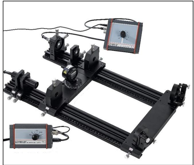
Fig. 14: Setup to measure the intensity distribution of a white LED lamp
