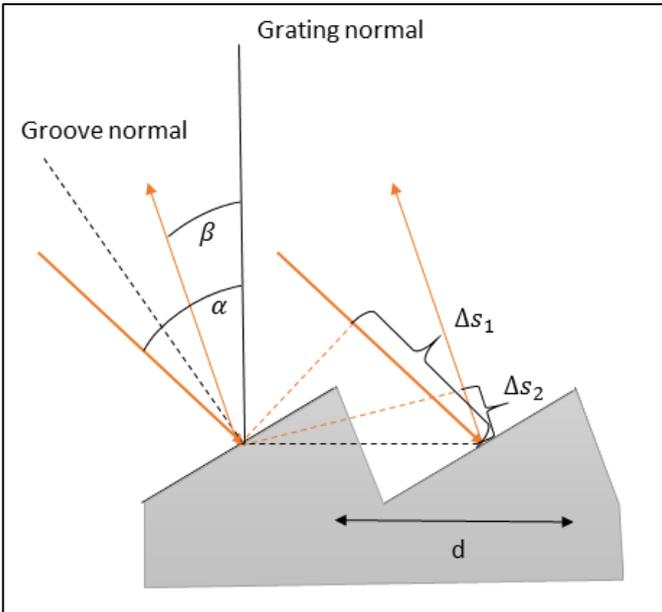
Fig. 2: The directions of diffracted orders for a reflective diffraction grating. Incident and reflected light are on the same side of the grating normal.
