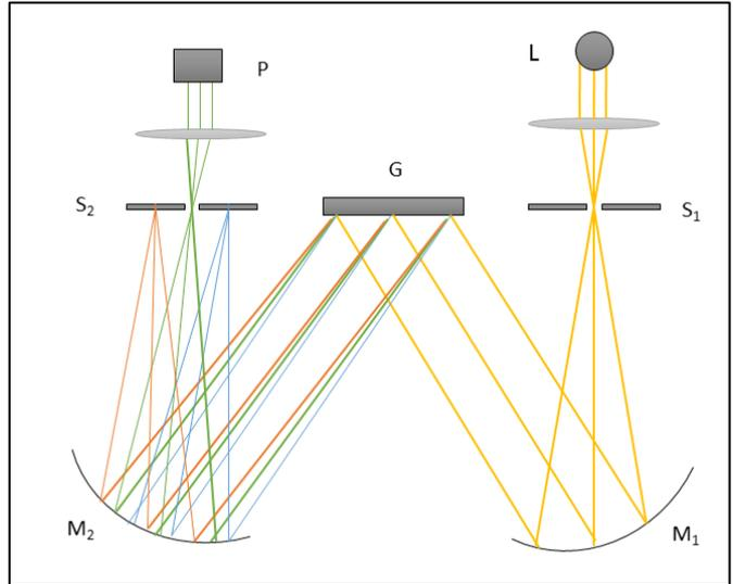
Fig. 3: Principle of a Czerny-Turner monochromator.
