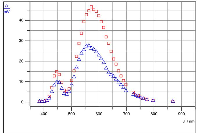
Fig. 17: Intensity distribution of the white LED with filter (blue) and without filter (red).
