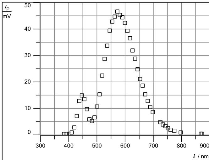
Fig. 15: Intensity distribution of a white LED.
