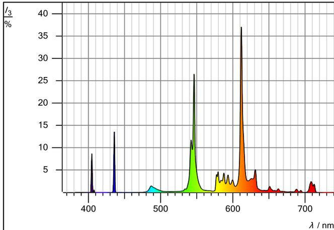
Fig. 4: Spectrum of a mercury lamp.
