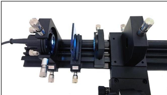
Fig. 16: Measuring the spectral properties of an acrylic absorption filter.
