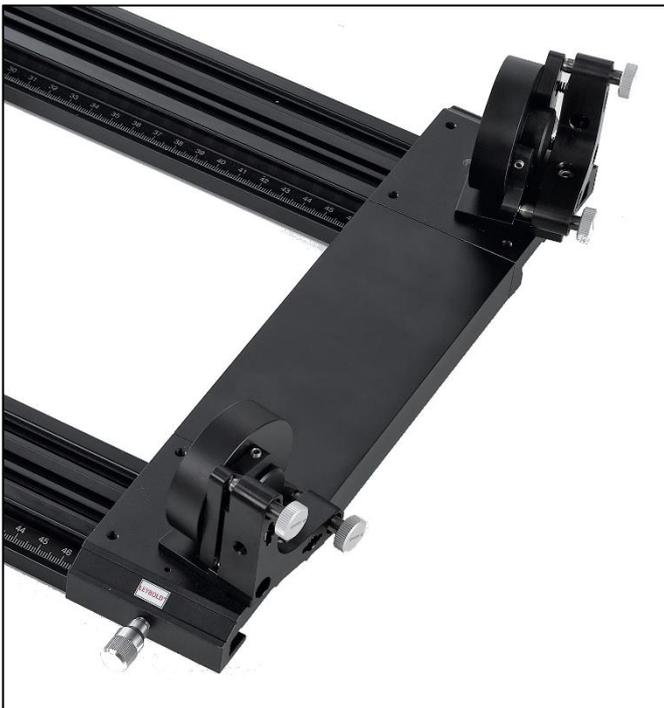
Fig. 7: Spectrometer Mirror Assembly mounted at the end of the profile rails.
