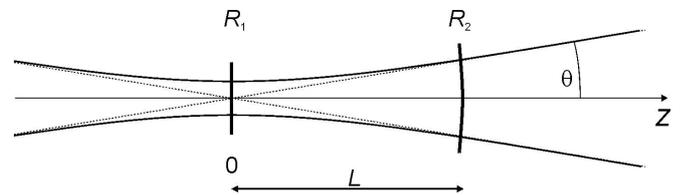
Fig. 2: Beam path for a resonator with  $R_1 \rightarrow \infty$
