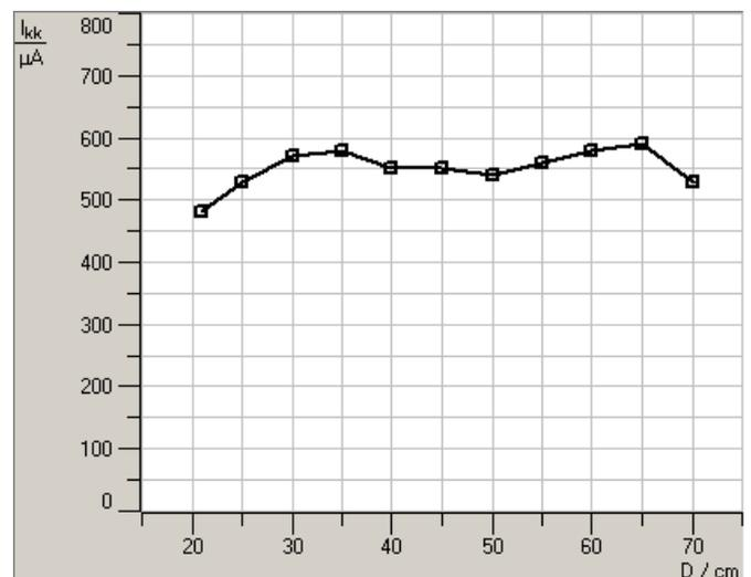
Fig. 5: Dependence of the output power on the laser tube position for  $R_1 = R_2 = 1000$  mm and  $L = 90$  cm
