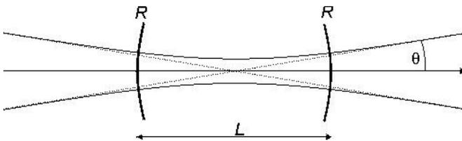
Fig. 1: Beam path for a resonator with  $R_1 = R_2 = R$
