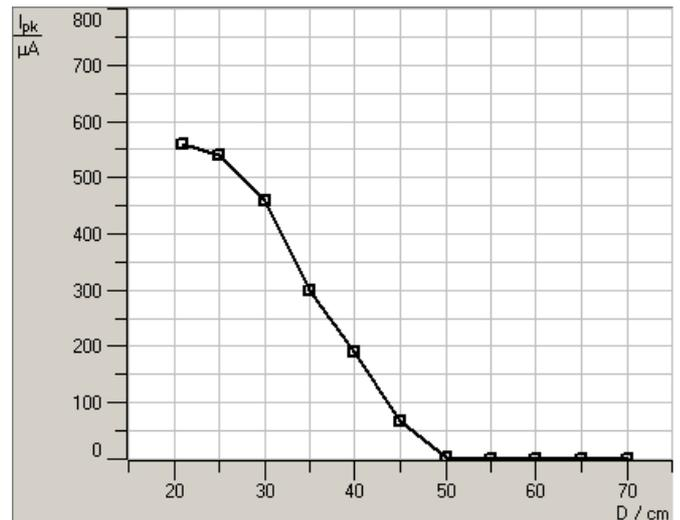
Fig. 4: Dependence of the output power on the laser tube position for  $R_1 \rightarrow \infty$ ,  $R_2 = 1000$  mm and  $L = 90$  cm
