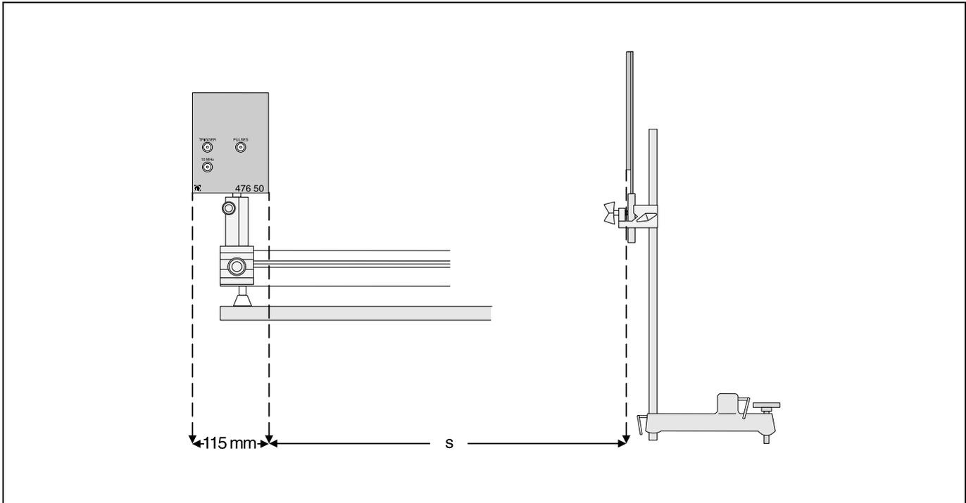
Fig. 4: Measuring the position of the light velocity measuring instrument and the large triple mirror
