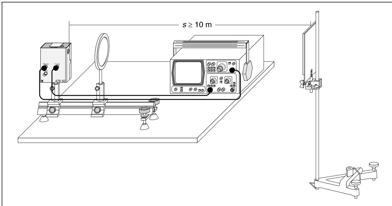
Fig. 2: Experiment setup for measuring the velocity of light
