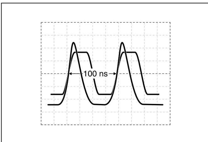
Fig. 6: Absolute measurement of the transit time  $t$  of the light pulse with externally calibrated time base
