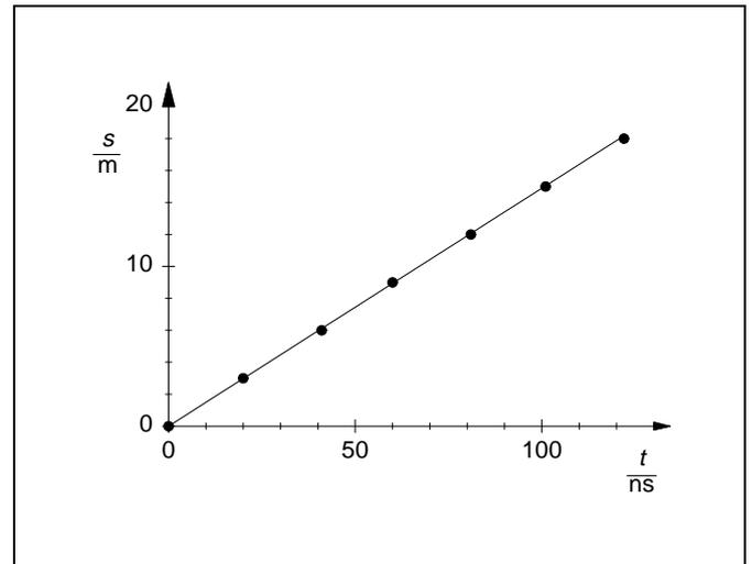
Fig. 7: Change in distance  $s$  of the large triple mirror as a function of the transit time  $t$  of the light pulse
