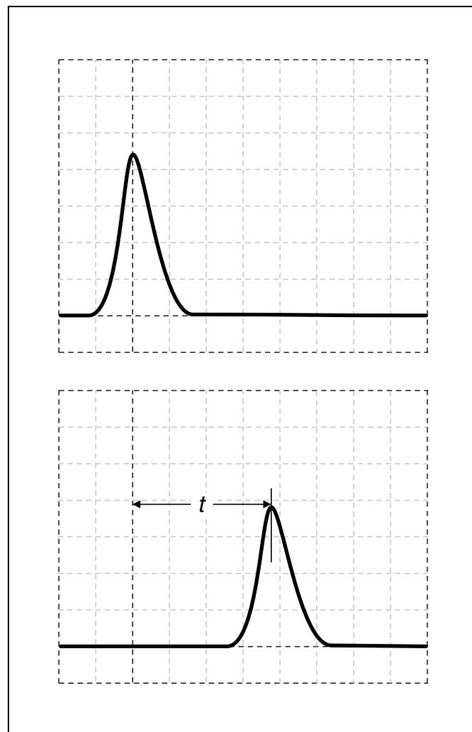
Fig. 3: Relative measurement of the transit time  $t$  of the light pulse
