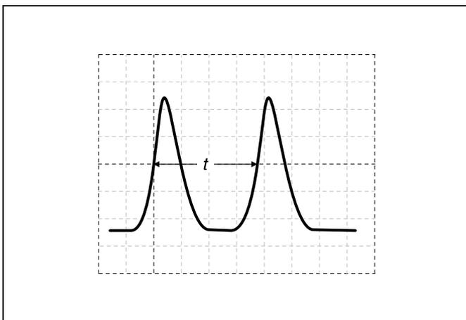
Fig. 5: Absolute measurement of the transit time  $t$  of the light pulse
