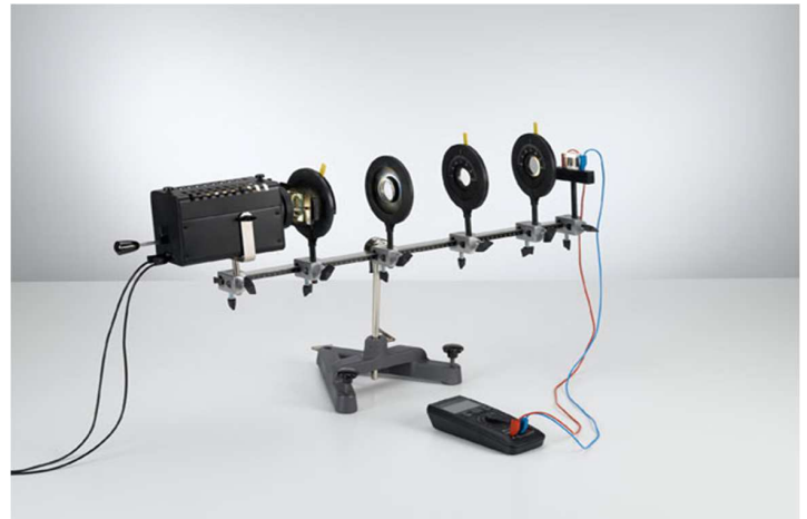
Figure 3: Experiment set-up, Malus' Law.
