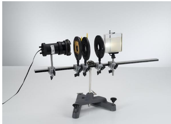
Figure 2: Experiment set-up, polarization of light by scattering in an emulsion.
