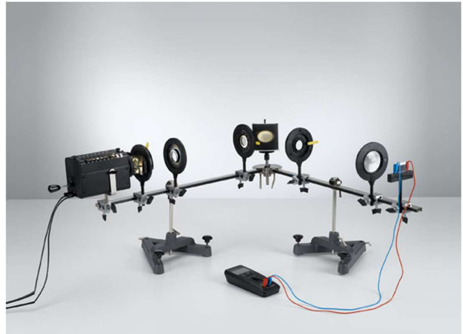
Figure 2: Experiment set-up, Fresnel's Laws of Reflection.
