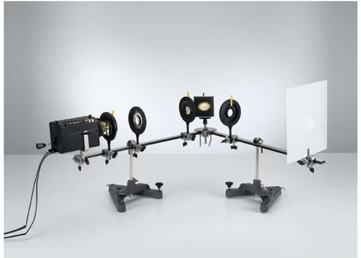
Figure 2: Experiment set-up, polarization of light by reflection on a glass plate.
