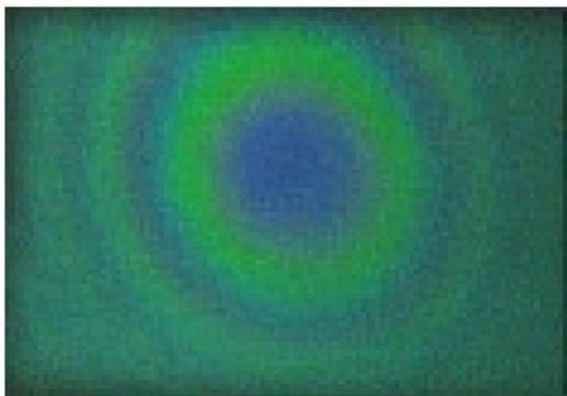
Fig. 3: Interference pattern on the screen without filter
