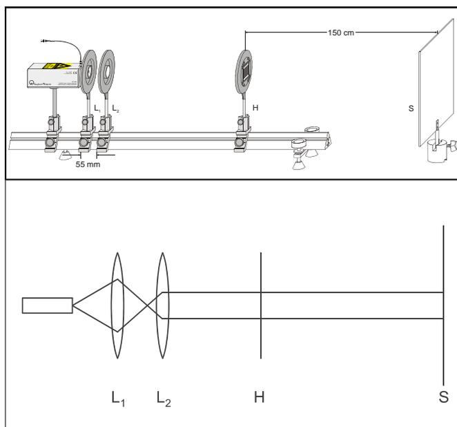
Fig. 4: Experimental setup for observing diffraction at a grating
