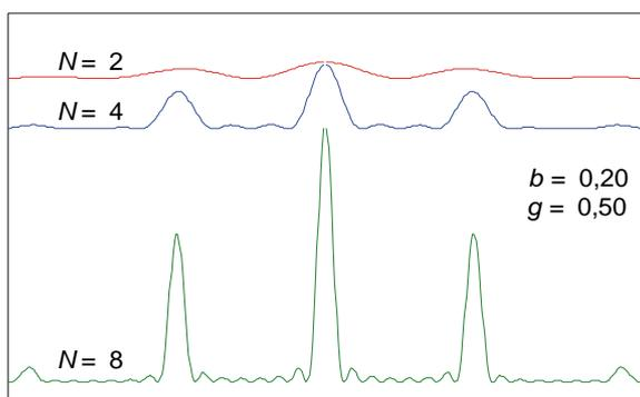
Fig. 2: Formation of the diffraction pattern of gratings starting from a double slit and then with increasing line number  $N$ . The intensity distributions shown have been calculated using equation (IV).
