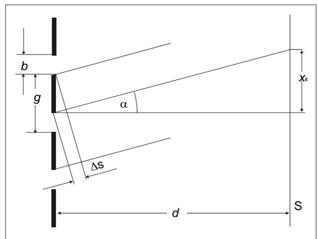
Fig. 1: Geometrical relations in the diffraction of light at a groove grating
