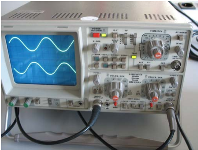
Fig. 4: Input signal (top of oscilloscope screen) and output signal (bottom top of oscilloscope screen) of the operational amplifier (inverting case).
