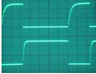
U_{CE} at the transistors T1 (top) and T2 (bottom)
