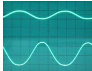
Illustration 5: Oscilloscope image when changing the voltage amplification top: input signal, bottom: output signal
