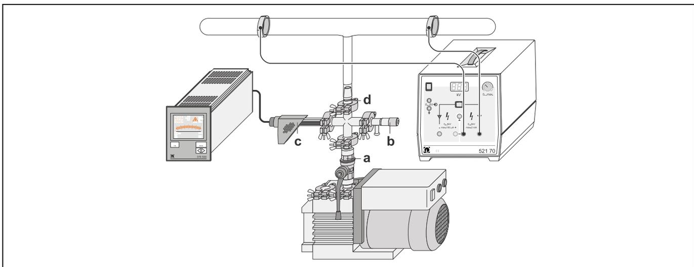
Fig. 3a  $p = 1013$  mbar: no discharge occurs ( $U = 5.0$  kV)
