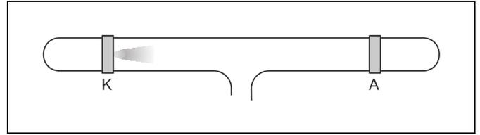
Fig. 3c  $p = 7$  mbar: the streamer becomes thicker (positive column), small luminous spot at the cathode, small dark space in front of the cathode ( $U = 1.1$  kV)
