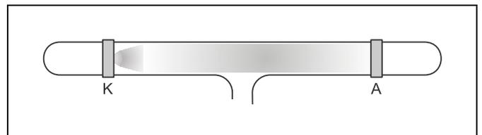
Fig. 3i  $p = 0.035$  mbar: glow light in front of the cathode disappears; in front of the anode fluorescence arises, and behind the cathode there is a luminous effect ( $U = 5.0$  kV)
