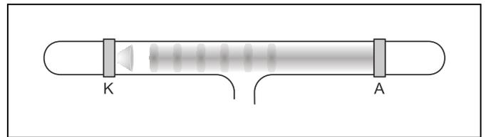
Fig. 3f  $p = 0.2$  mbar: diffuse light at the cathode, large dark space, positive column: distance between layers increases ( $U = 0.7$  kV)
