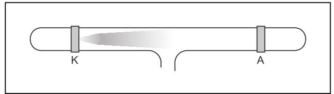
Fig. 3d  $p = 0.8$  mbar: the whole cathode is covered with a luminous layer; dark space between cathode and the positive column widens ( $U = 0.8$  kV)
