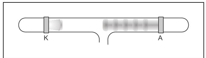
Fig. 3h  $p = 0.06$  mbar: glow light in front of the cathode expands, and the positive column disappears ( $U = 1.8$  kV)
