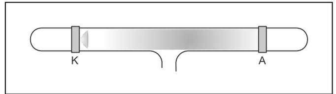
Fig. 3e  $p = 0.35$  mbar: positive column loses colour, and bright and dark zones emerge ( $U = 0.6$  kV)
