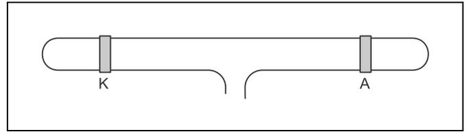
Fig. 3b  $p = 40$  mbar: small luminous cone in front of the cathode (blue-red streamer from the cathode to the anode,  $U = 2.6$  kV)
