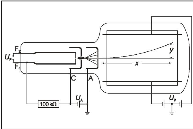
Fig. 2: Deflection in an electric field
