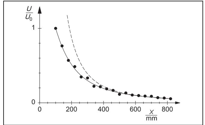
Fig. 6 Longitudinal distribution of the normalized received signal in front of the horn antenna
