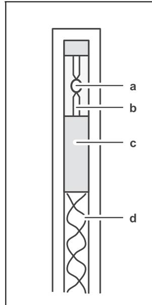
Fig. 2 Internal structure of the E-field probe
