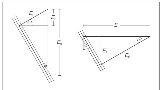
Fig. 8 Calculation of the components of the electric field
