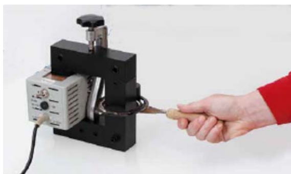
Fig. 1: Melting tin in an induction oven.
