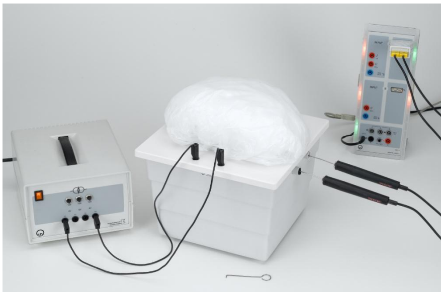
Fig. 1. Determination of the thermal conductivity of a building material sample using the single-plate method.
