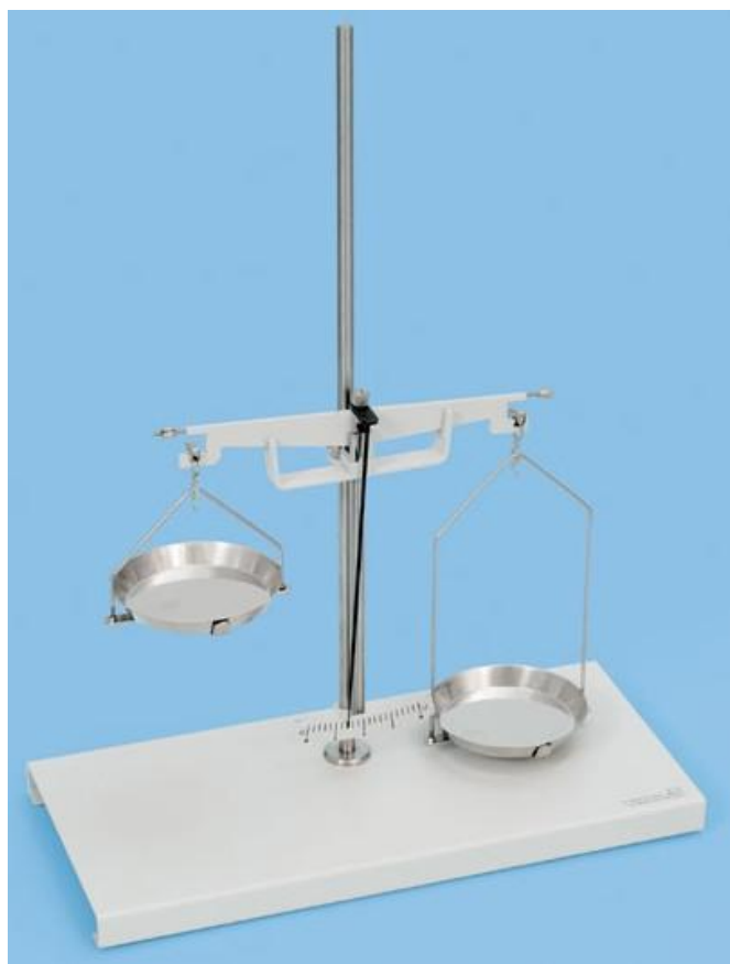
Fig.1: Hydrostatic balance with one short arm and one long arm.
