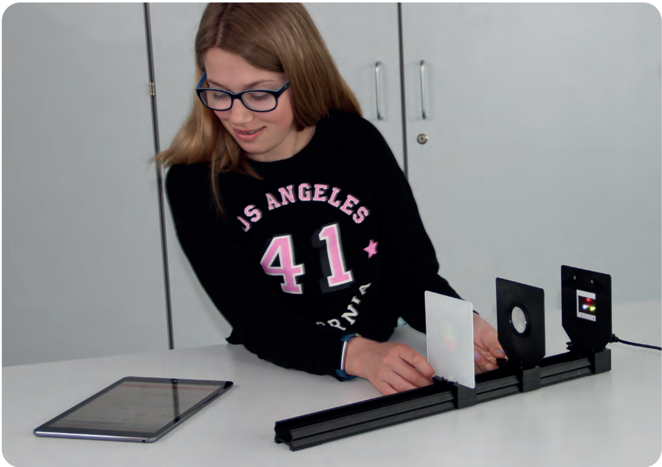
LP5.2.3.4 Additive mixing of three light colours
