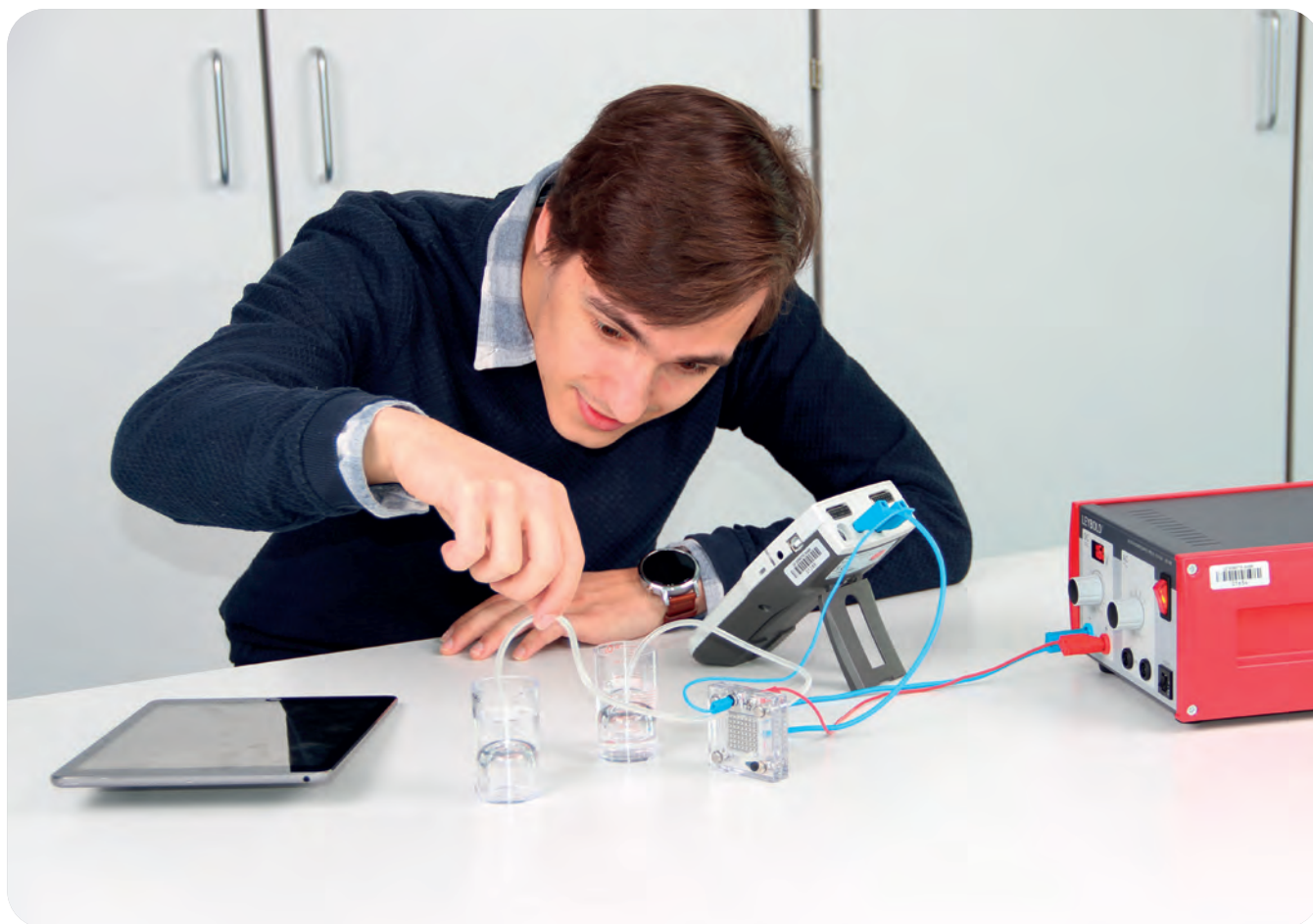
LP2.3.2.1 Using a reversible fuel cell as an electrolyser
