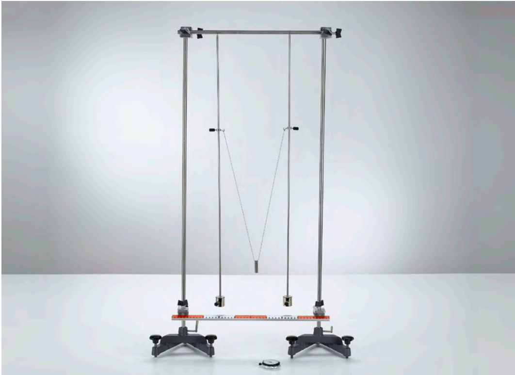
Coupled pendulum - Measuring with a hand-held stopclock (P1.5.4.1)
