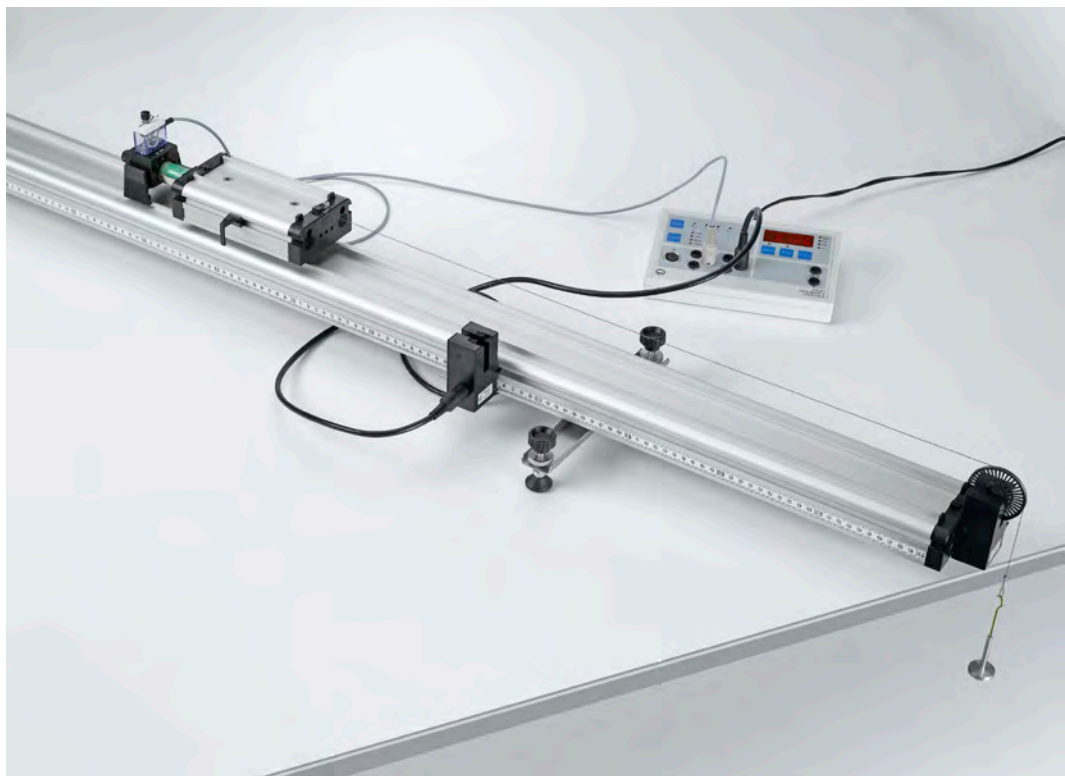
Path-time diagram of straight motion - Recording the time with a counter (P1.3.2.1)
