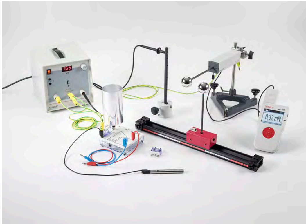
Confirming Coulomb's law - Measuring with the force sensor (P3.1.2.2)
