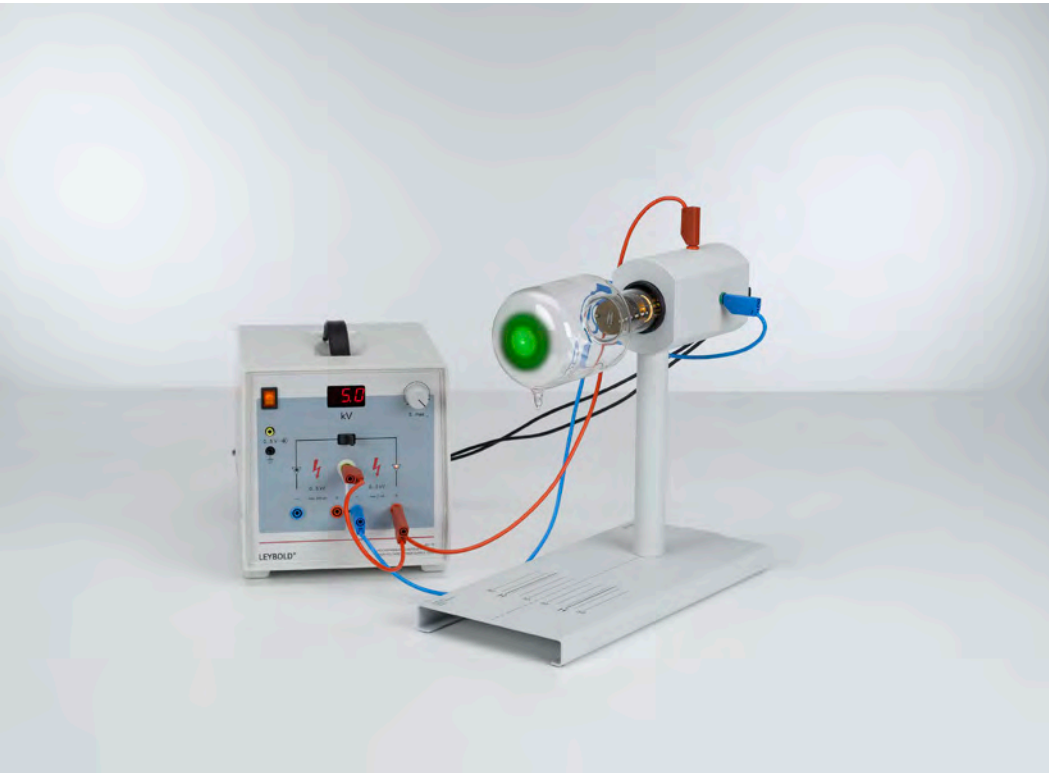
Diffraction of electrons at a polycrystalline lattice (Debye-Scherrer diffraction) (P6.1.5.1)
