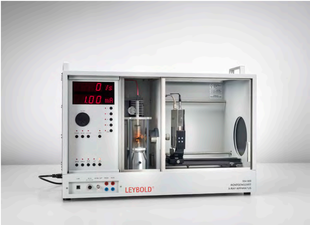
Digital Laue diagrams: investigating the lattice structure of monocrystals (P7.1.2.5)
