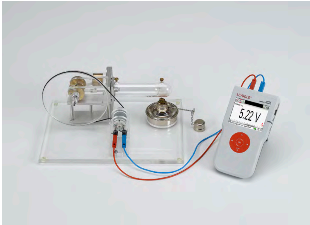
Operating the hot-air engine P as a thermal engine, heat pump and a refrigerator (P2.6.1.5)
