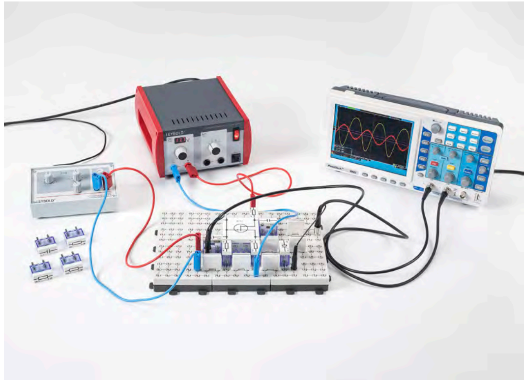
The field-effect transistor as an amplifier (P4.1.6.5)
