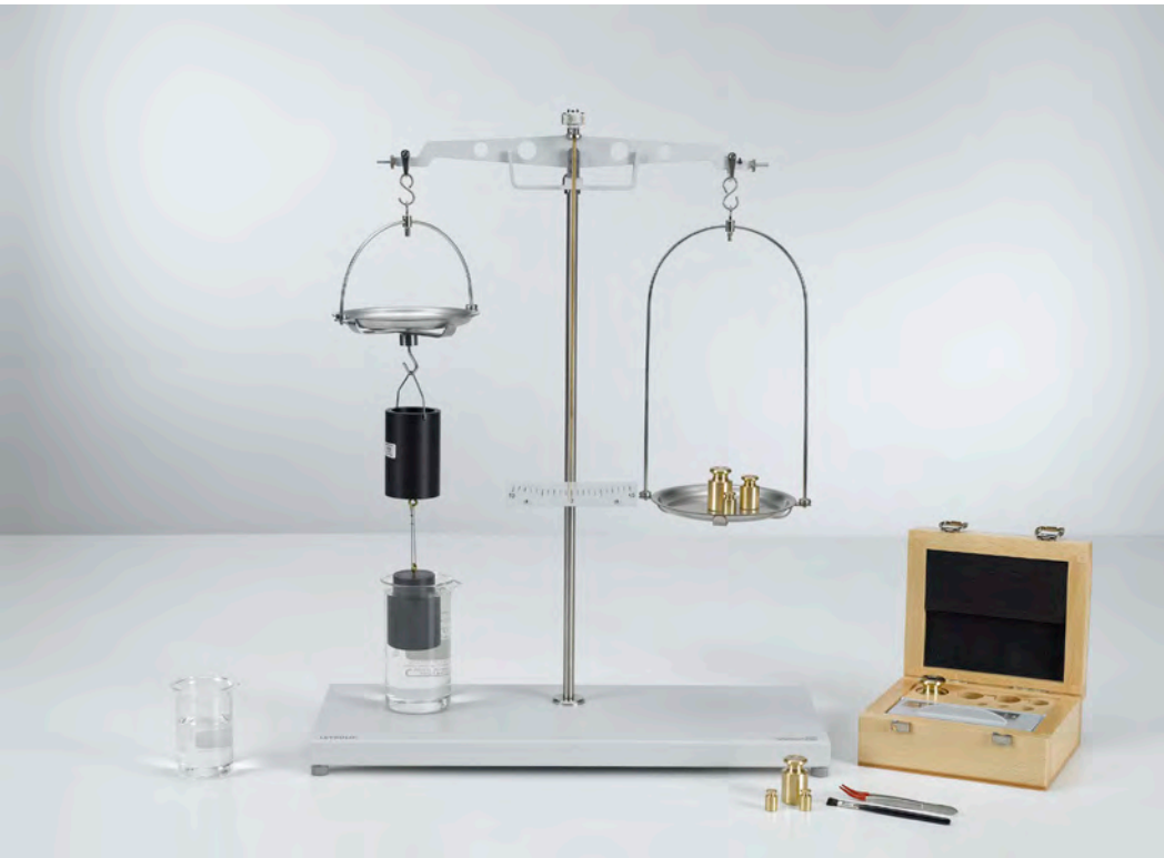
Confirming Archimedes' principle (P1.8.2.1)
