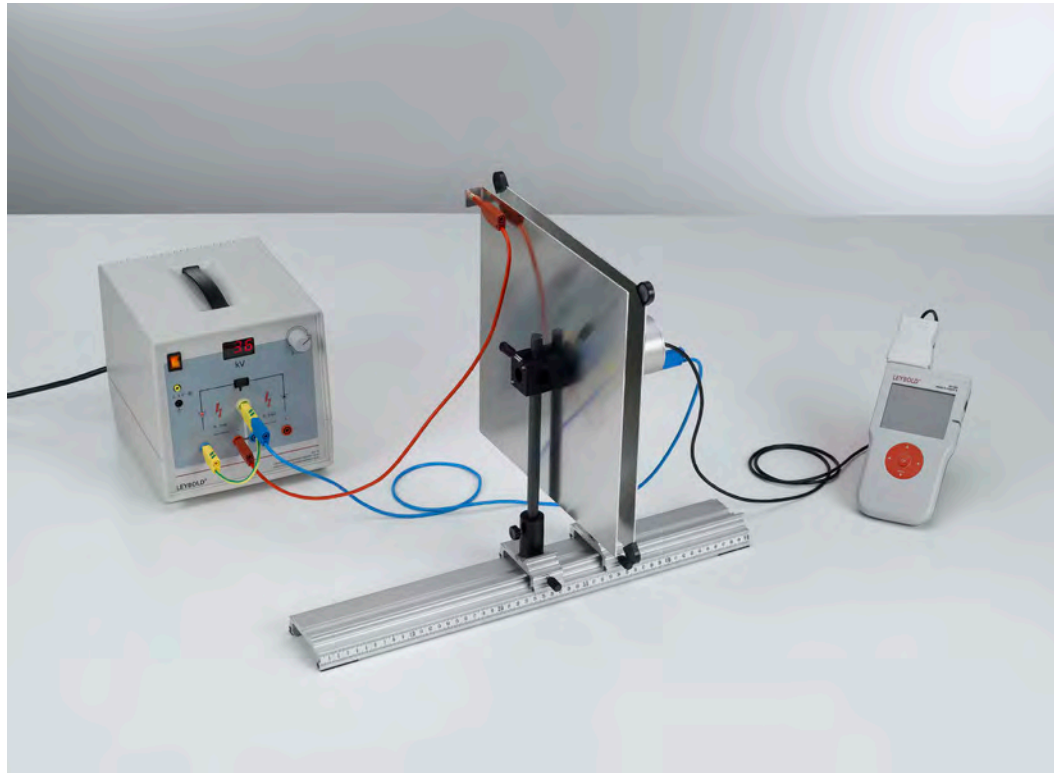
Measuring the electric field strength inside a plate capacitor (P3.1.7.4)
