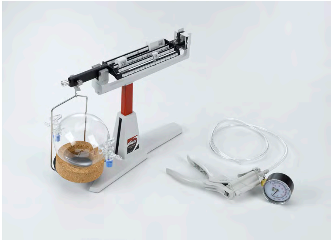
Determining the density of air (P1.1.2.4)
