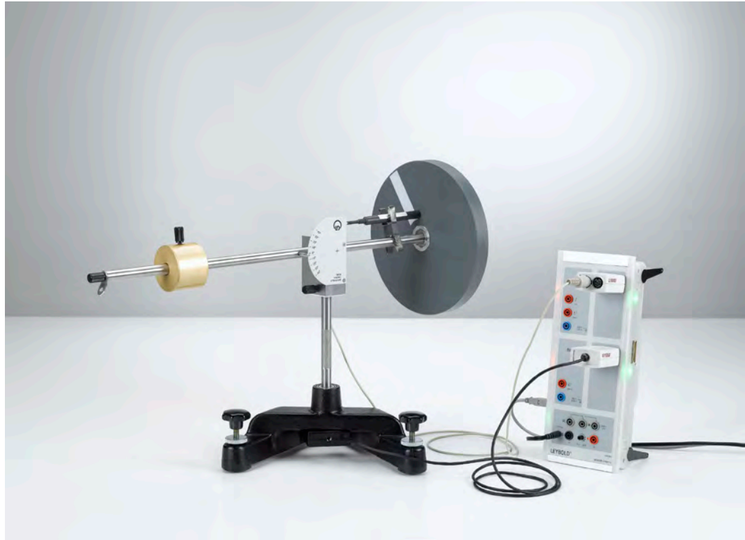
Precession and nutation of a gyroscope (P1.4.4.3)
