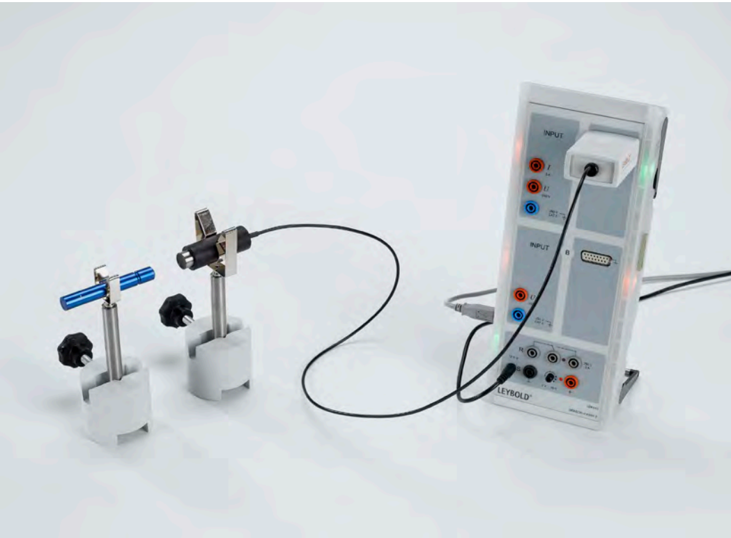
Statistical variations in determining counting rates (P6.4.2.1)
