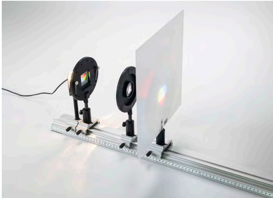
Demonstration of additive color mixing (P5.2.3.2)
