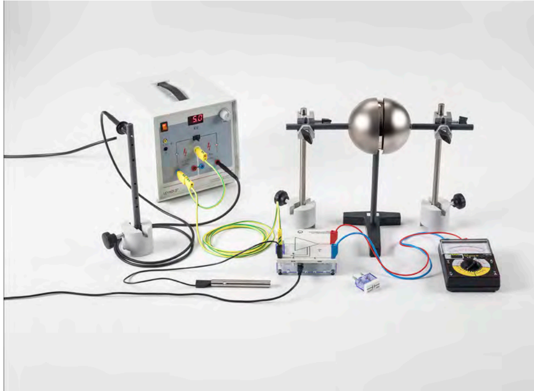
Electrostatic induction with the hemispheres according to Cavendish (P3.1.5.2)
