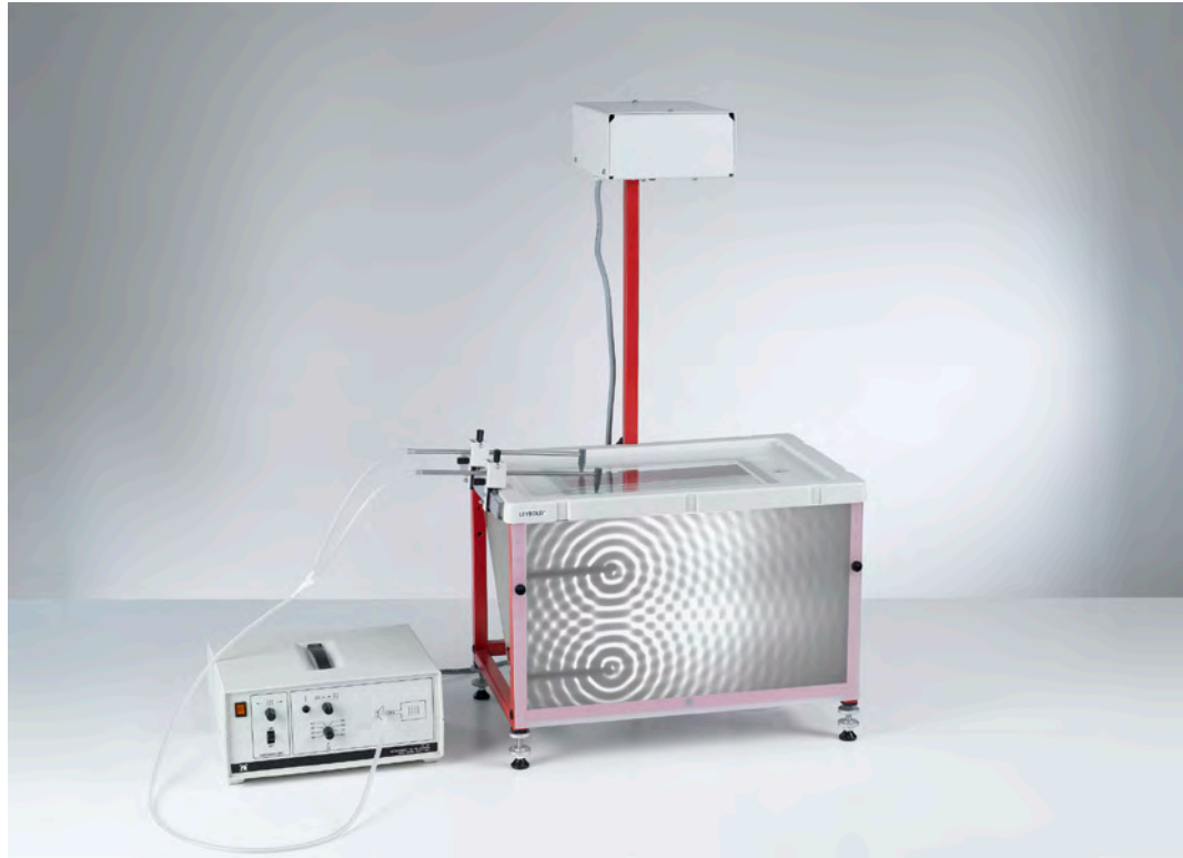
Two-beam interference of water waves (P1.6.5.1)
