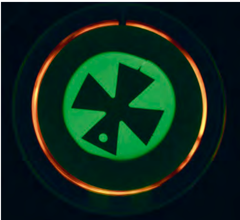
Shadow of the maltese cross on the fluorescent screen (P3.8.3.1)
