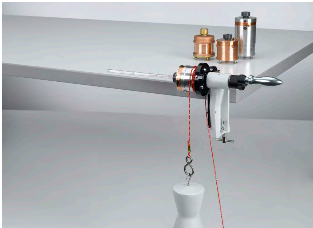
Converting mechanical energy into heat energy - Recording and evaluating measured values manually (P2.3.3.1)
