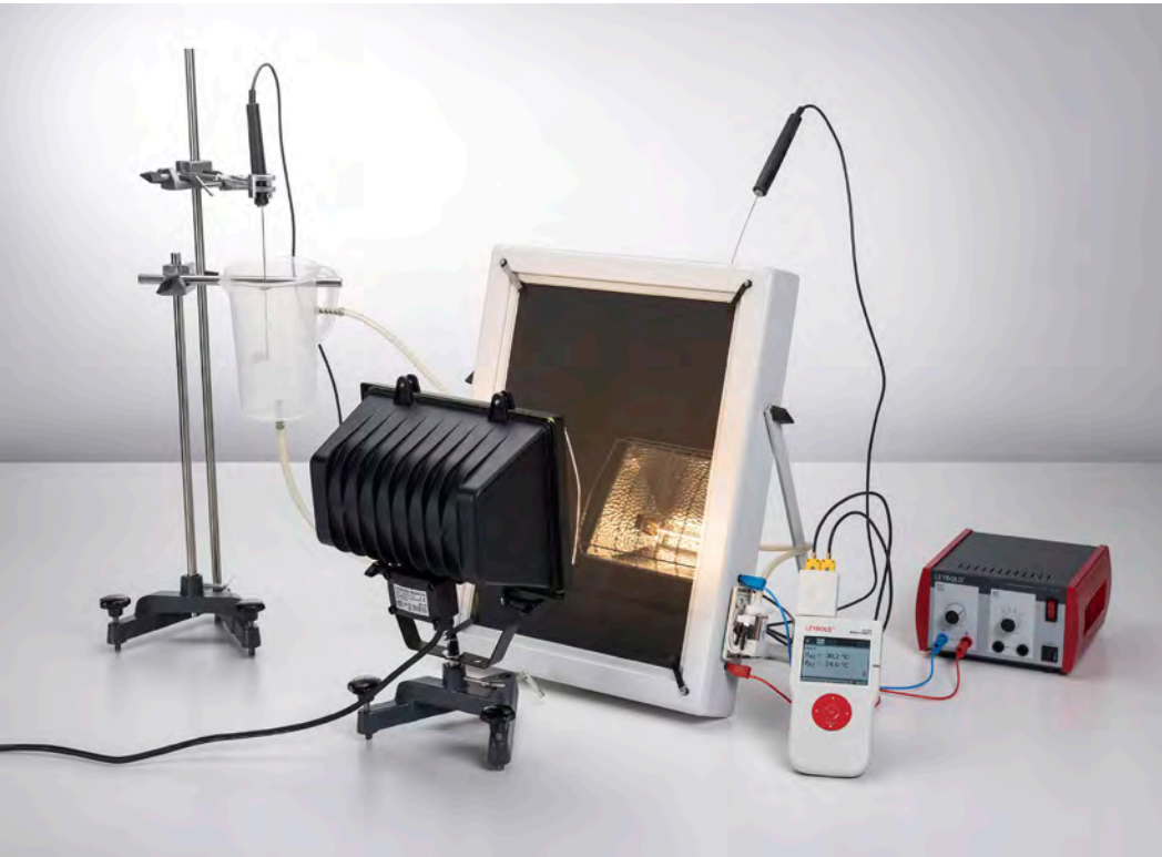
Efficiency of a solar collector (P2.2.2.1)
