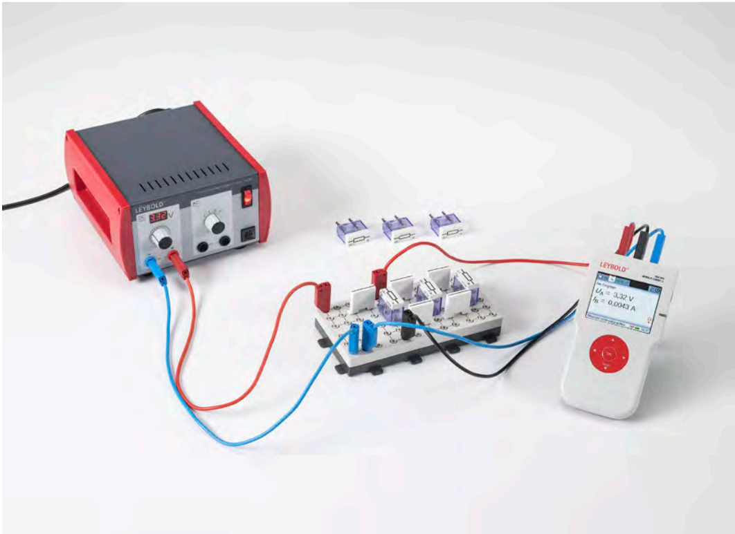
Measuring current and voltage at resistors connected in parallel and in series (P3.2.3.1)
