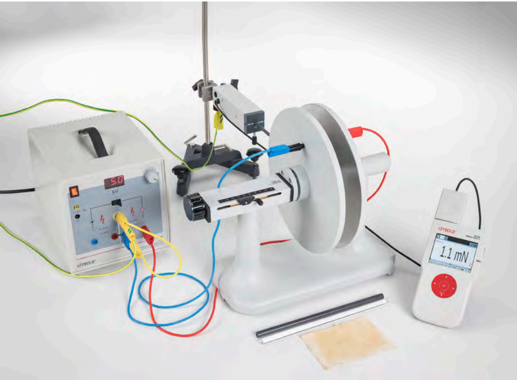
Measuring the force of an electric charge in a homogeneous electric field - Measuring with the force sensor (P3.1.4.4)
