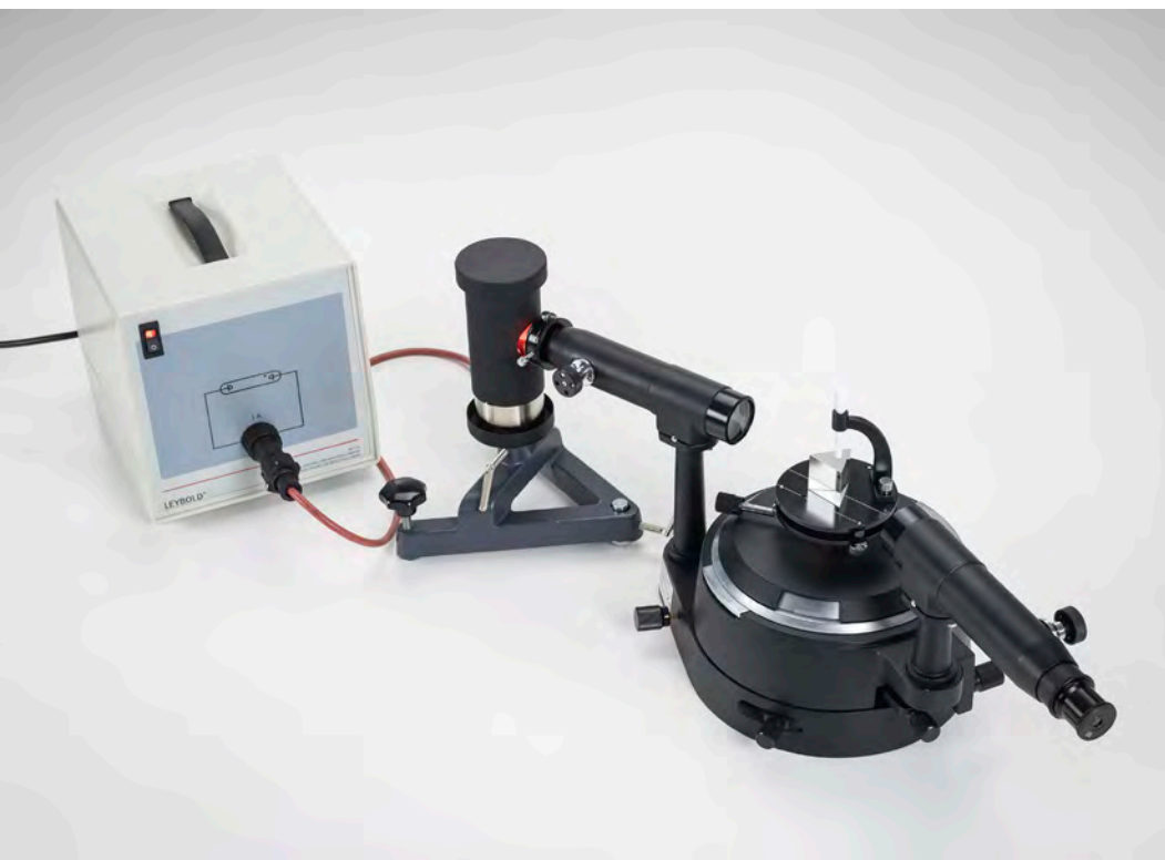
Measuring the line spectra of inert gases and metal vapors using a prism spectrometer (P5.7.1.1)
