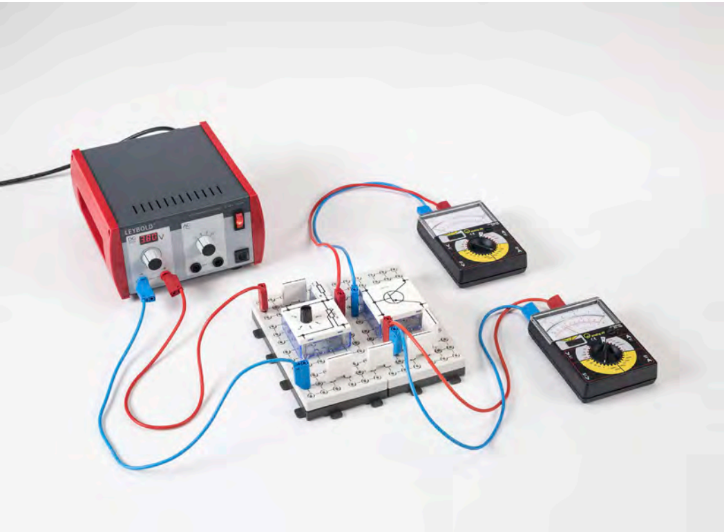
Recording the characteristics of a transistor (P4.1.5.2)
