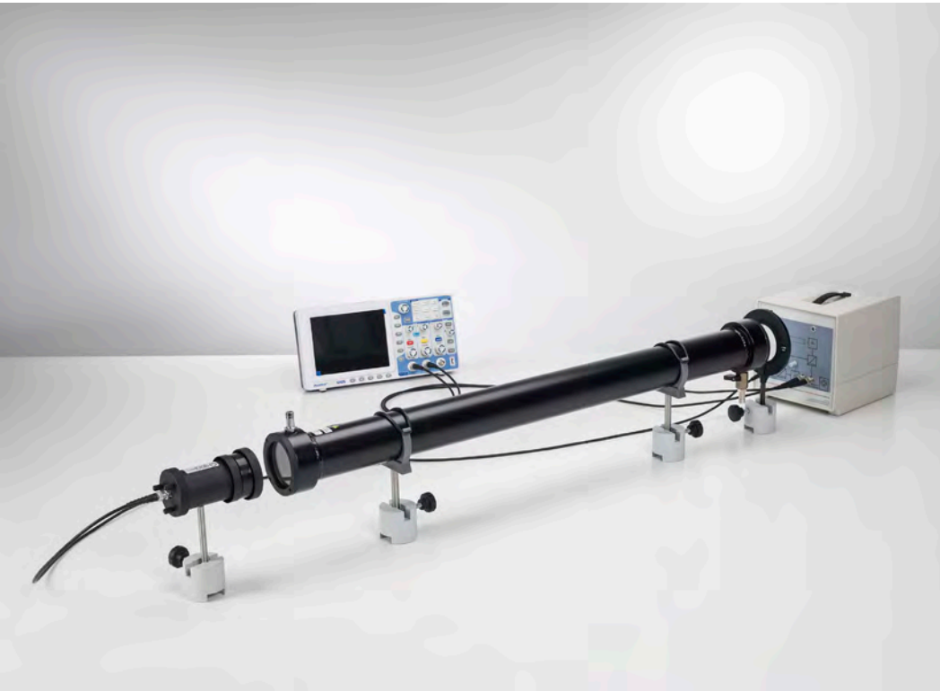
Determining the velocity of light in various materials (P5.6.3.2)
