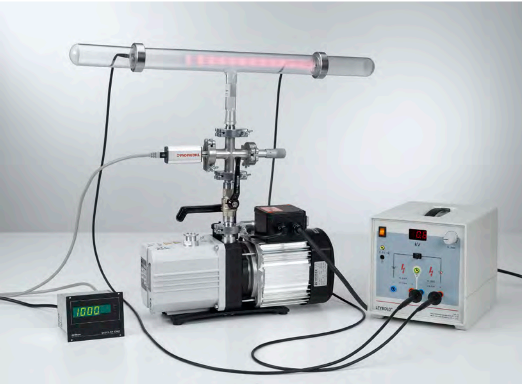
Investigating spontaneous gas discharge in air as a function of pressure (P3.9.2.1)
