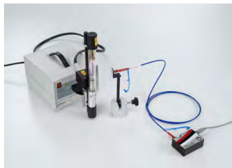
Emission spectrum of atomic hydrogen (P6.2.1.4)
