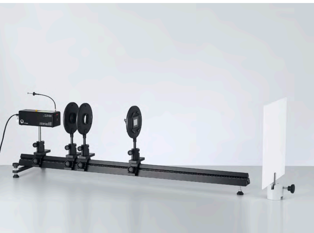
Diffraction at a double slit and multiple slits (P5.3.1.2)
