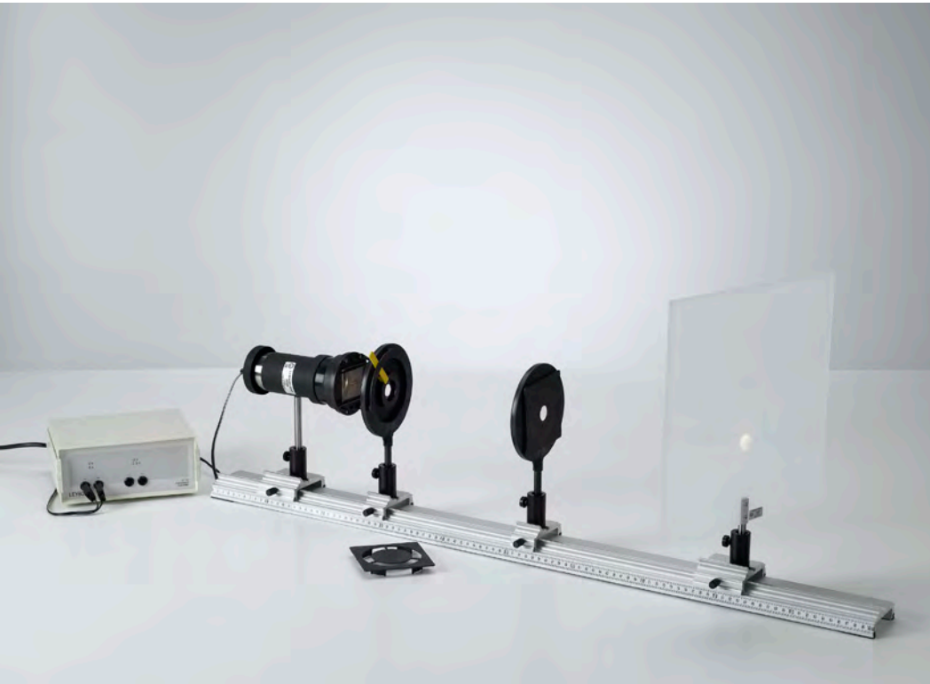
Spherical aberration in lens imaging (P5.1.3.1)
