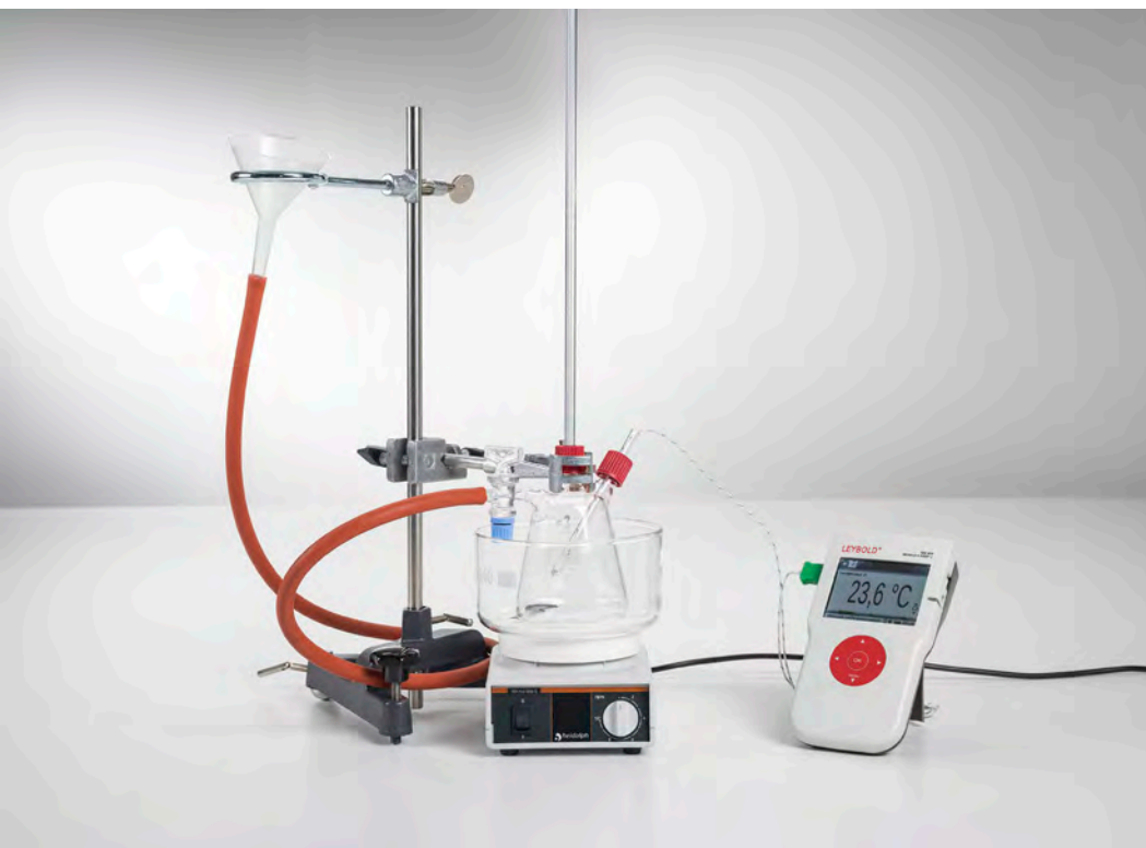
Investigation of the density maximum of water - Measuring with Mobile-CASSY (P2.1.3.2)
