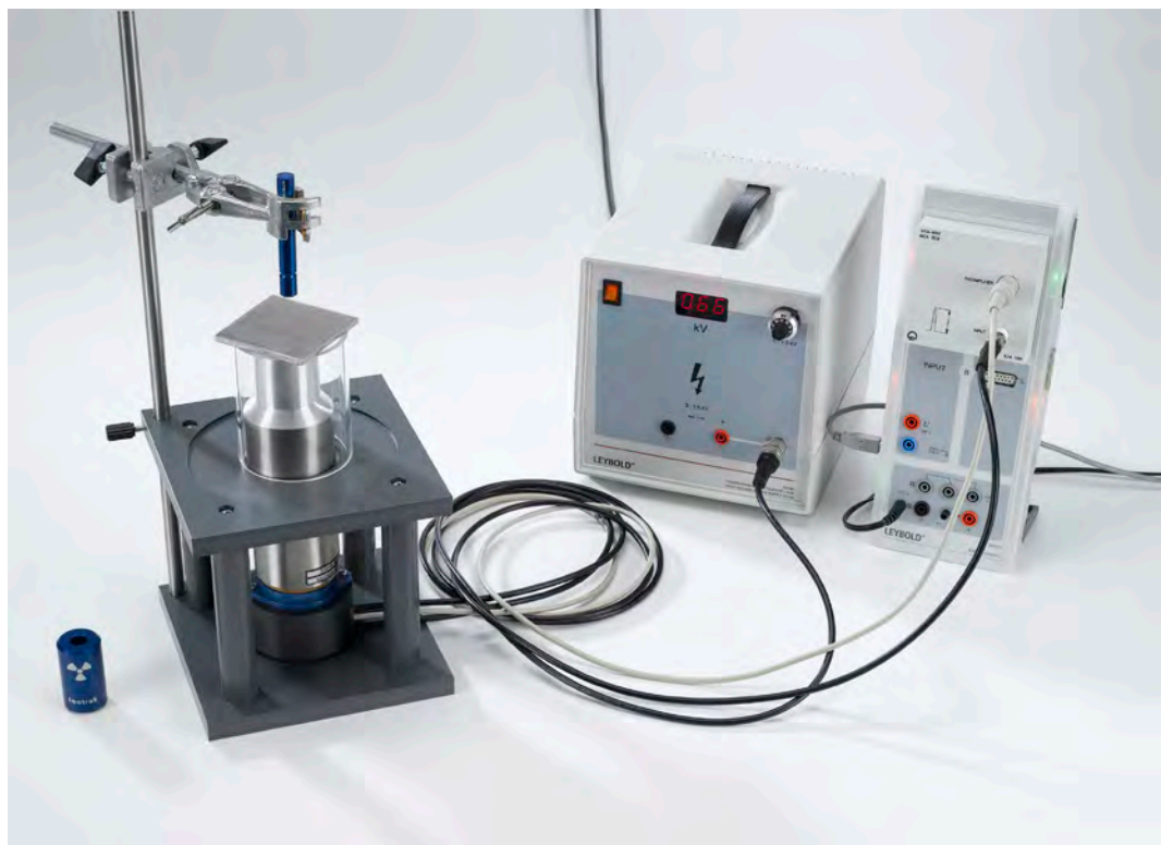
Absorption of \gamma radiation (P6.5.5.3)
