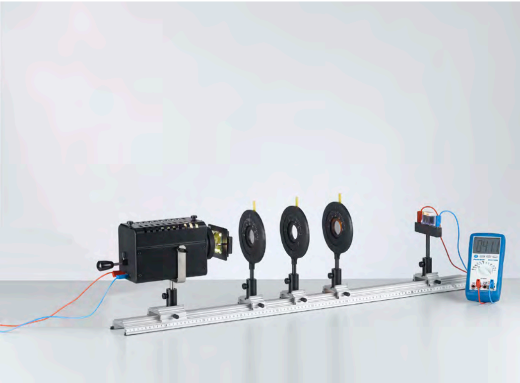
Quarter-wavelength and half-wavelength plate (P5.4.2.2)
