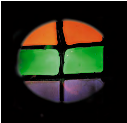
Exciting luminescence through irradiation with ultraviolet light and electrons (P7.2.4.1)
