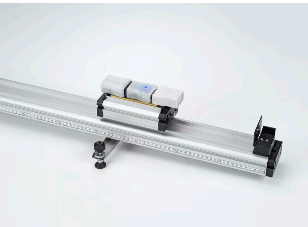
Accelerated motions with an acceleration sensor (P1.3.2.5)
