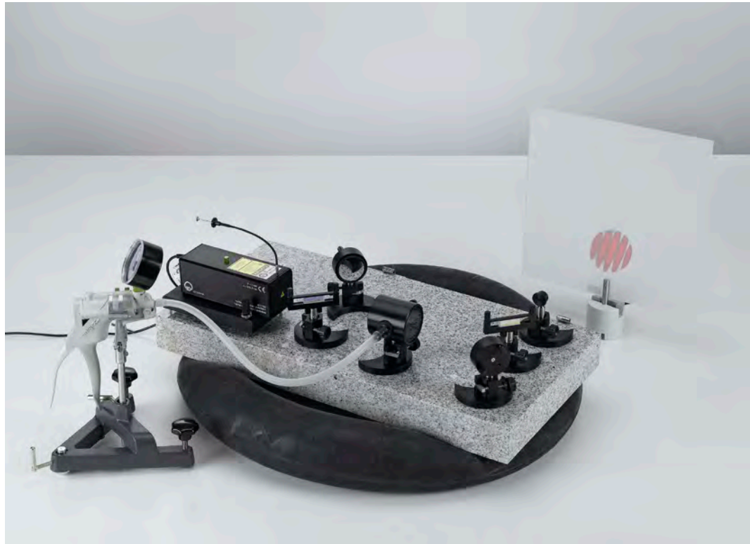
Measuring the refractive index of air with a Mach-Zehnder interferometer (P5.3.5.2)
