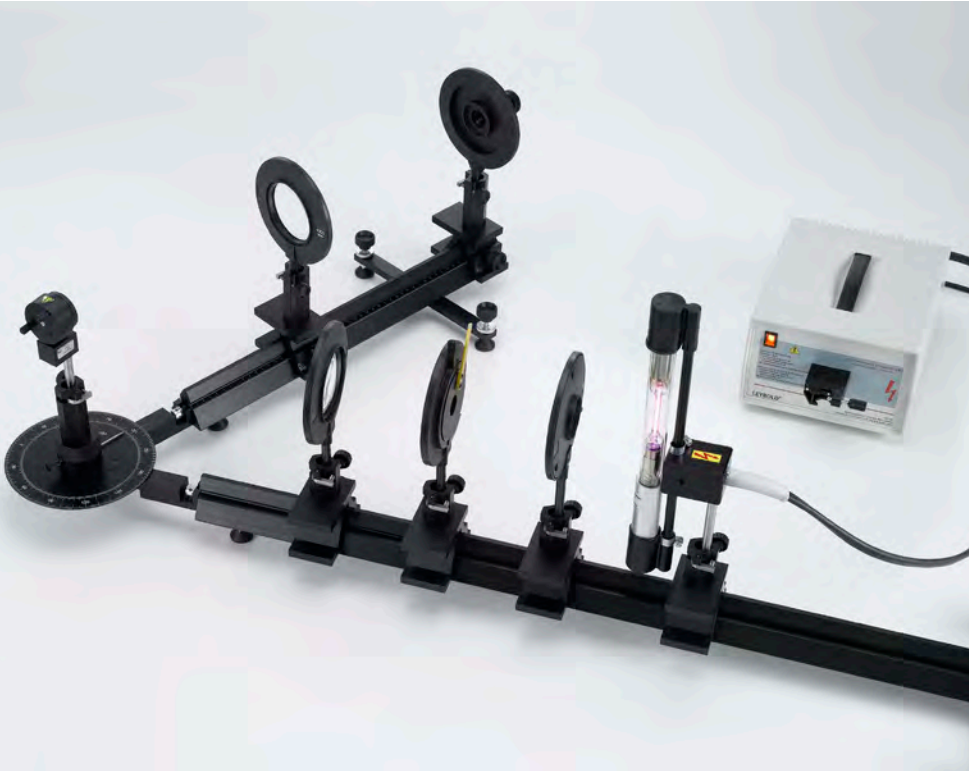
Observing the splitting of the Balmer series on deuterated hydrogen (isotope splitting) - Observing the line splitting with a telescope setup (P6.2.1.5)
