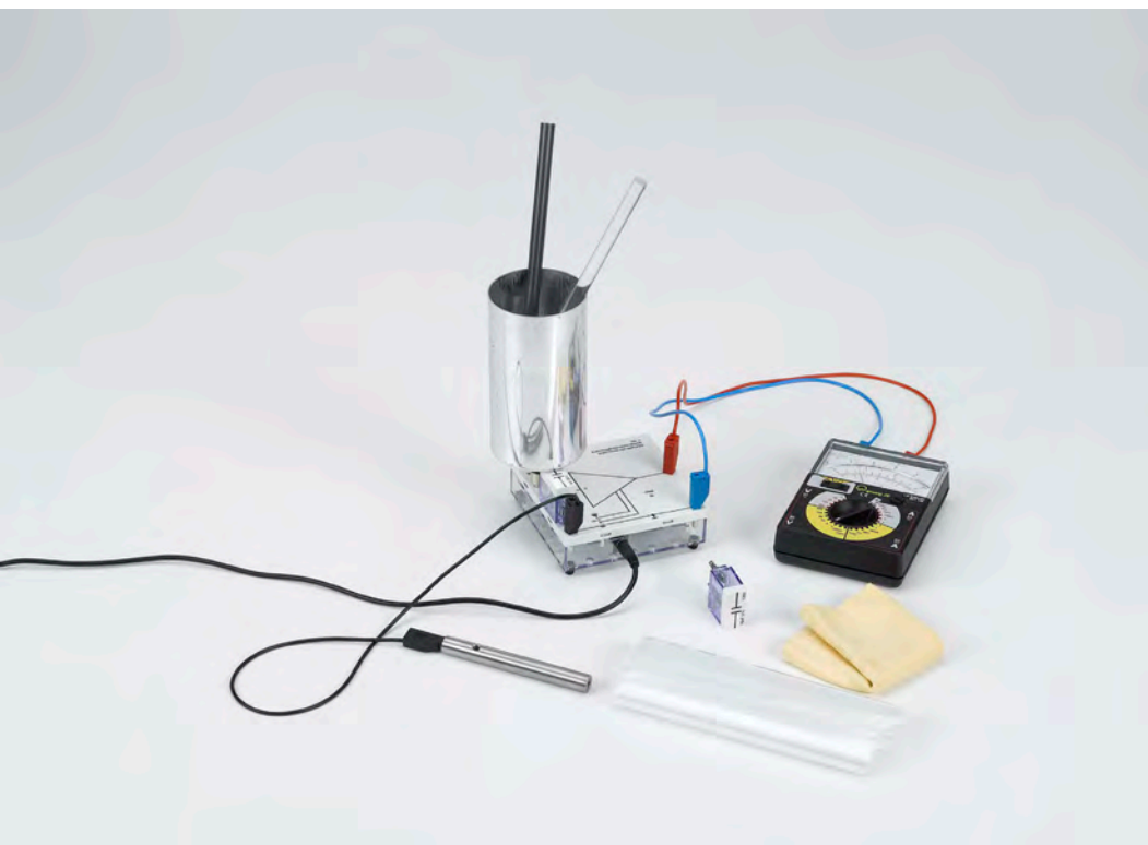
Basic electrostatics experiments with the electrometer amplifier (P3.1.1.2)
