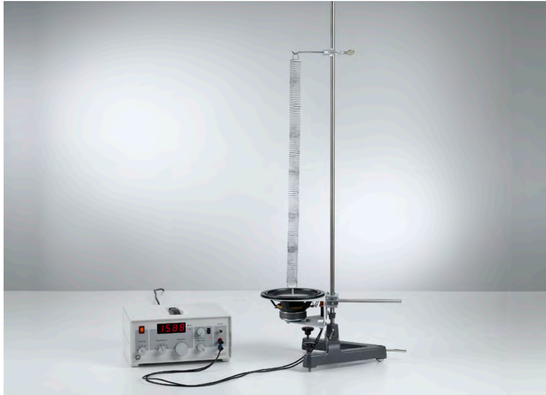
Production of standing waves on a helical spring and determination the wavelength (P1.6.1.5)
