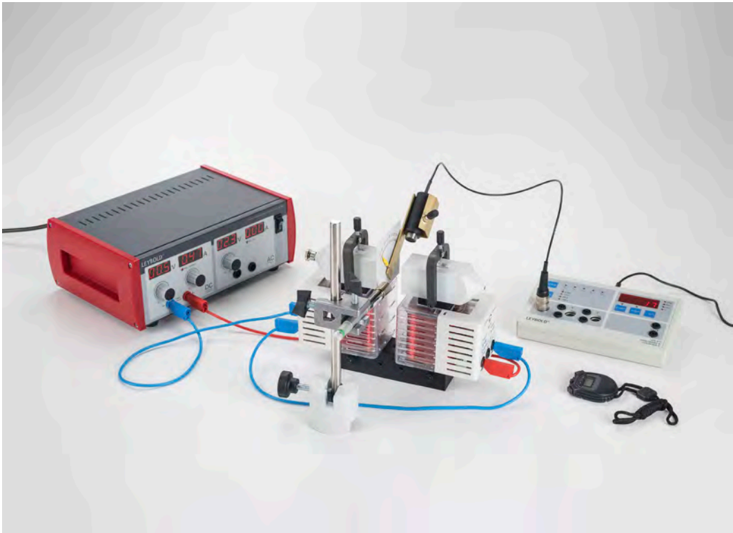
Deflection of beta radiation in a magnetic field (P6.5.7.1)
