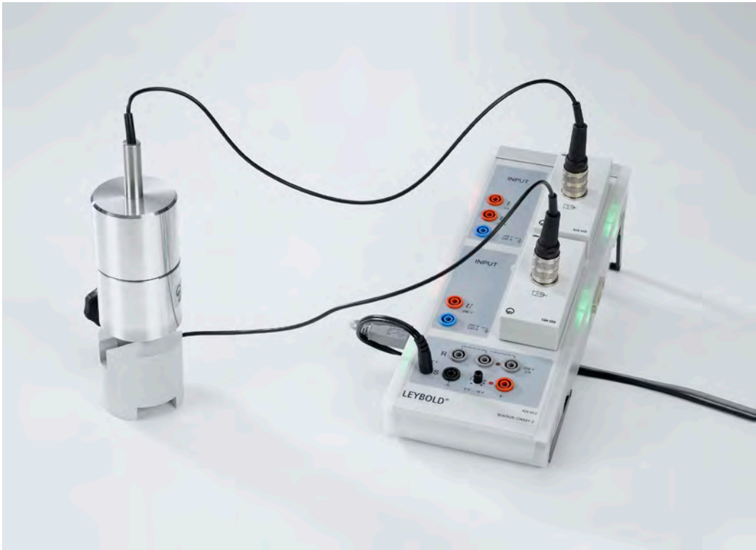
Detection of Muons (P6.6.2.1)
