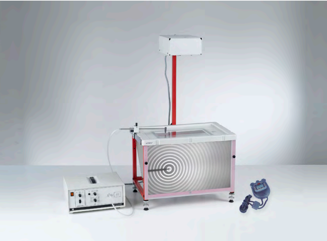
Exciting circular and straight water waves (P1.6.4.1)
