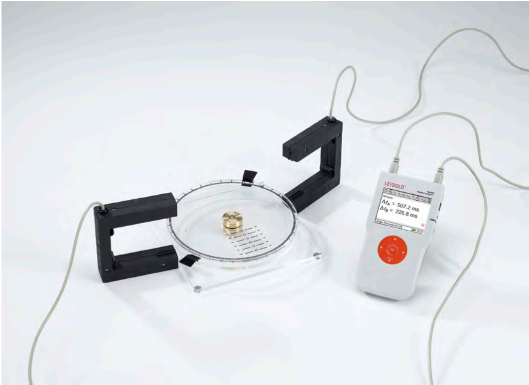
Conservation of angular momentum in elastic and inelastic rotational collision (P1.4.2.1)
