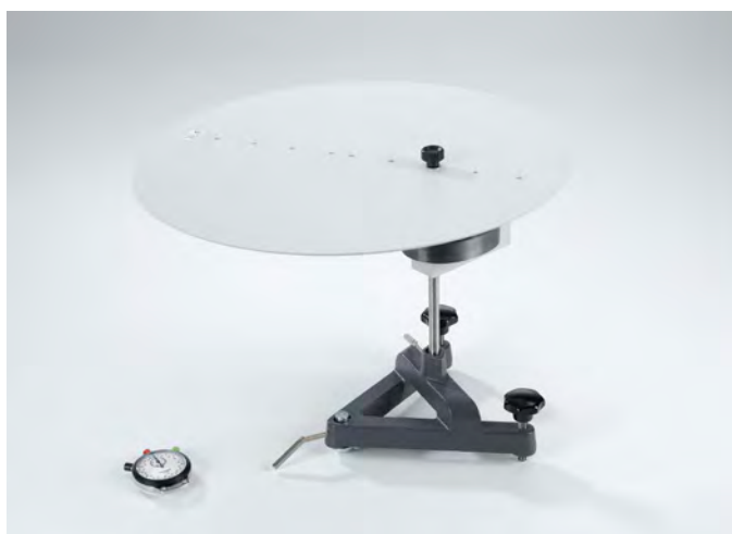
Confirming Steiner's theorem (P1.4.5.3)
