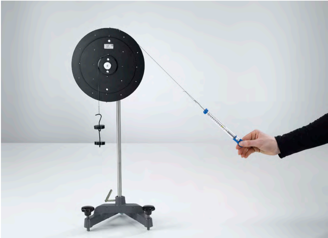
Wheel and axle as a lever with unequal sides (P1.2.3.2)
