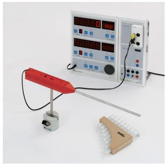
Microphone settings: Output signal: pulse  $\Pi$ Gain: maximum
