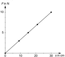
At a helical spring, the acting force and the spring elongation are proportional:  $F \sim s$ .
