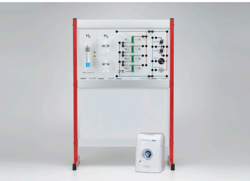
Investigation of a PEM fuel cell stack (C4.4.7.1)
