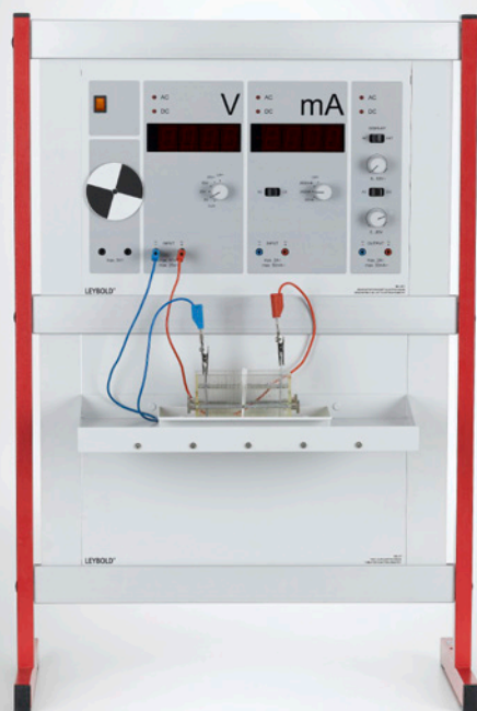
Standard potentials of metals (C4.4.3.2_a)
