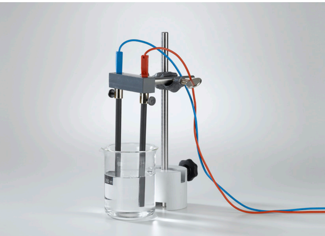
Electrolytic polarisation (C4.4.5.1)
