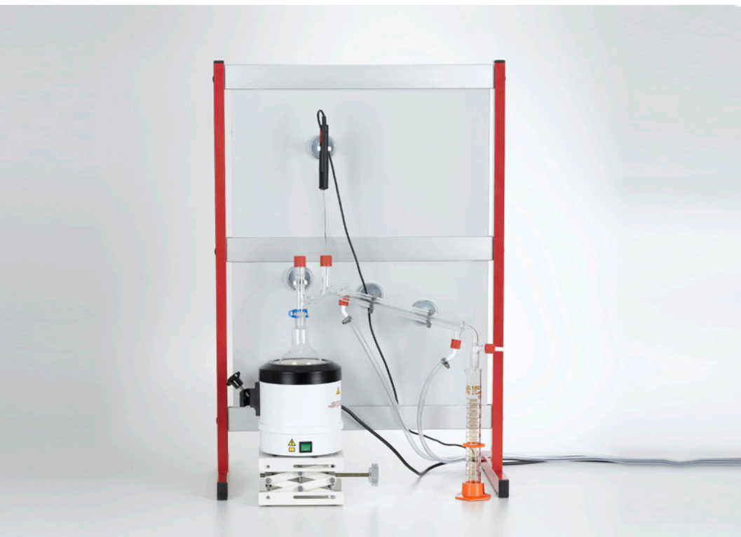
Boiling range distribution of petrol (C2.3.3.1)
