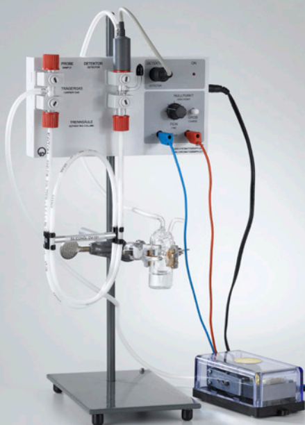
Gas chromatographical analysis of cigarette lighter gas (butane gas) (C3.2.1.1)
