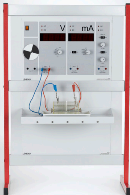
Concentration potentials (Nernst equation) (C4.4.3.4)
