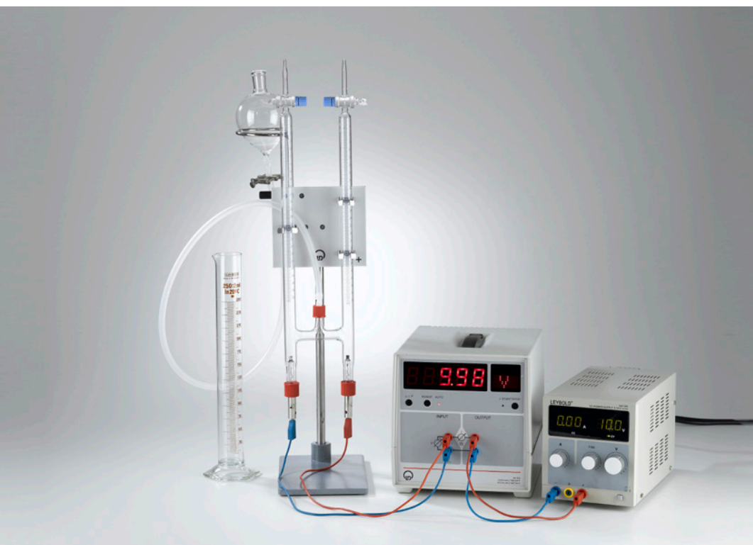
Determination of the Faraday constant (C4.4.5.2)
