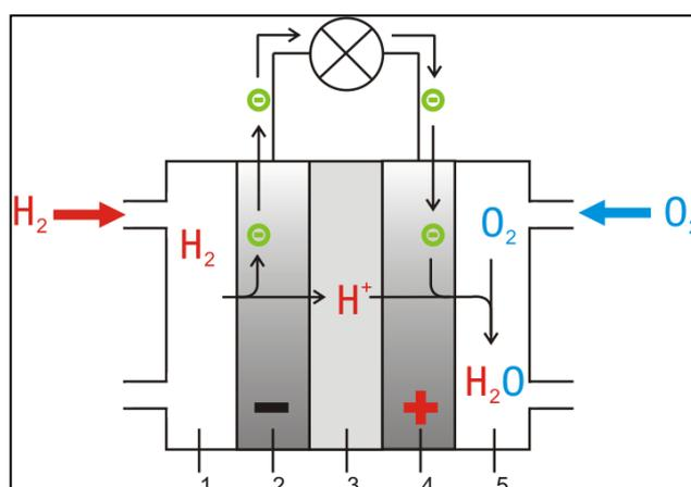
**Fig. 1: Model of a fuel cell.** 1 – H<sub>2</sub> chamber, 2 – Anode with catalyst, 3 – PEM (proton exchange membrane), 4 – Cathode with catalyst, 5 – O<sub>2</sub> chamber.
