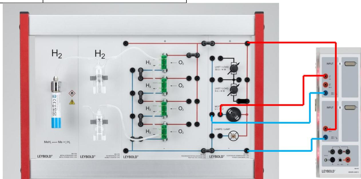
**Fig. 2** Experimental set-up for investigation of the fuel cell stack. The fuel cells are connected in series. Blue and red lines: Connections from the CPS module "Electric Load" to the Sensor-CASSY 2 using connecting leads. In this example, the motor is connected.
