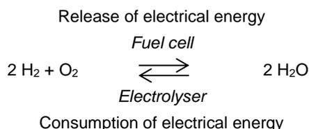
During the reaction of hydrogen with oxygen, energy is released. If one ignites the two substances directly, the energy is released in a large detonation. However, this energy can be converted directly into electrical energy using an appropriately constructed fuel cell (see Fig. 1). Decisive for this is having a suitable catalyst.
