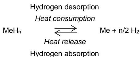
In this experiment, hydrogen is produced electrolytically and stored as a metal hydride. The fuel cells then to be investigated will be fed with hydrogen from the metal hydride storage container.
