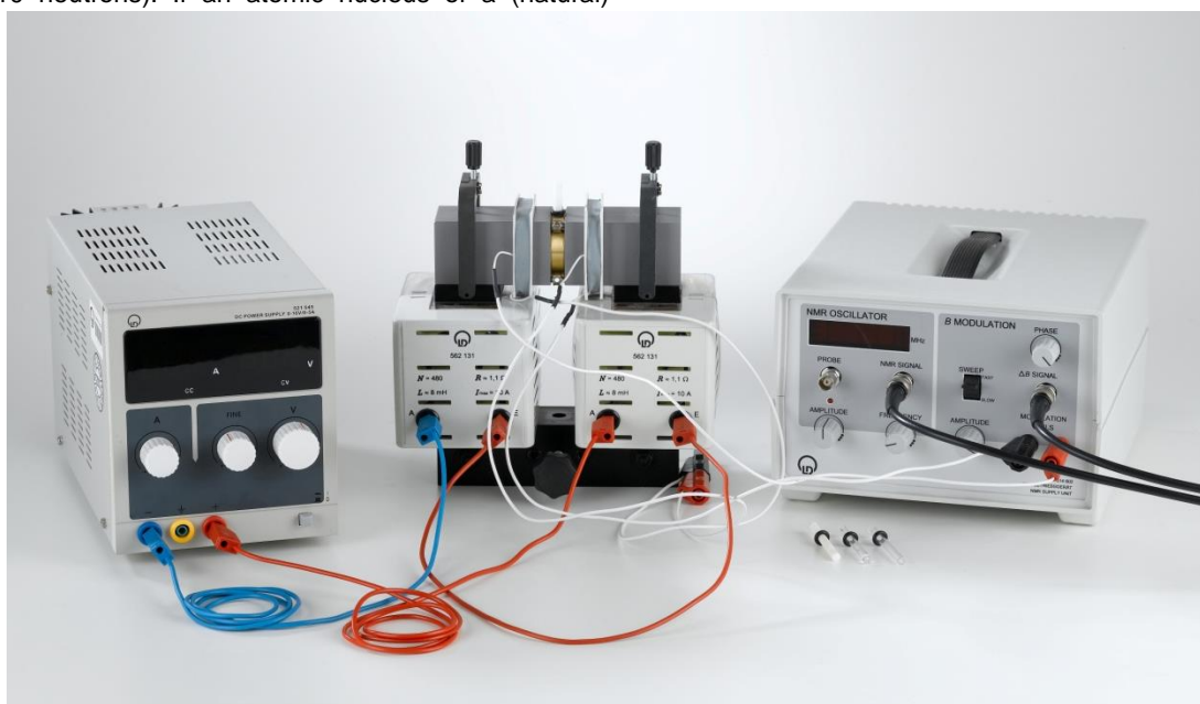
Fig. 1: Set-up of the experiment with power supply unit (DC power supply) for the electromagnets (on the left), NMR apparatus (in the middle) and NMR operating unit (on the right).
