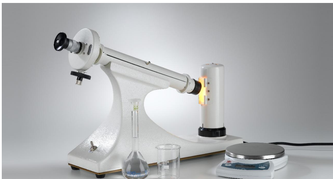
Fig. 1: Experimental apparatus for determining the rotation of the polarisation plane through sugar solution.
