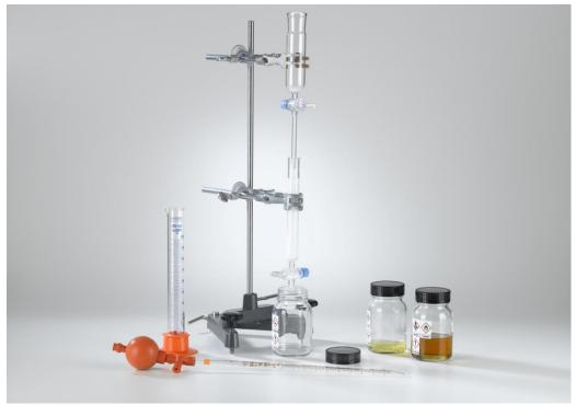
Fig. 1: Experimental apparatus for column chromatography with crude oil
