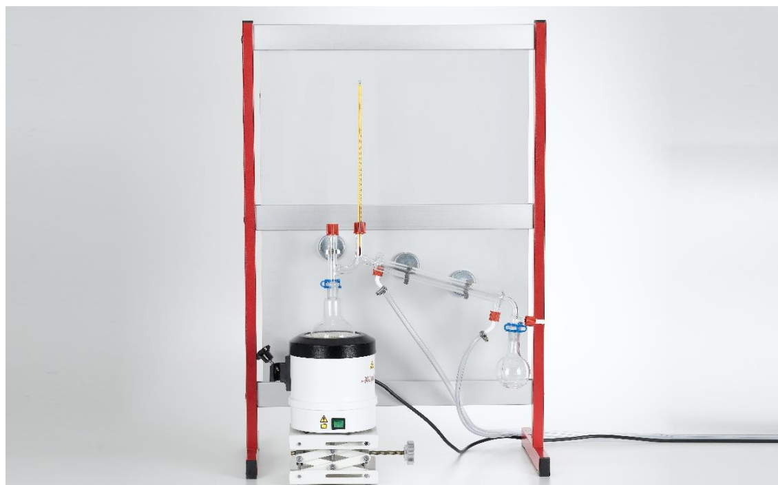
Fig. 1: Experiment apparatus for water vapour distillation.
