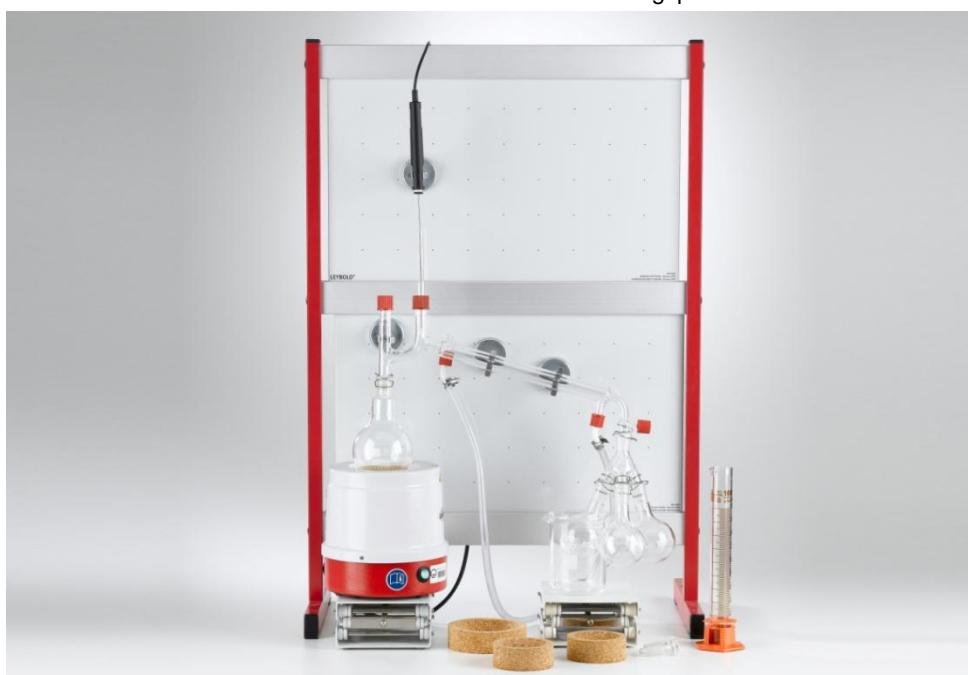
Fig. 1: Experimental apparatus for the distillation of crude oil.
