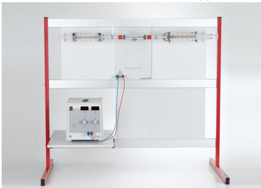
Fig. 1: Construction of the experiment. The gas syringes can also be attached with one large and one small magnetic holder each. Then affix the tube with the small magnetic holders.
