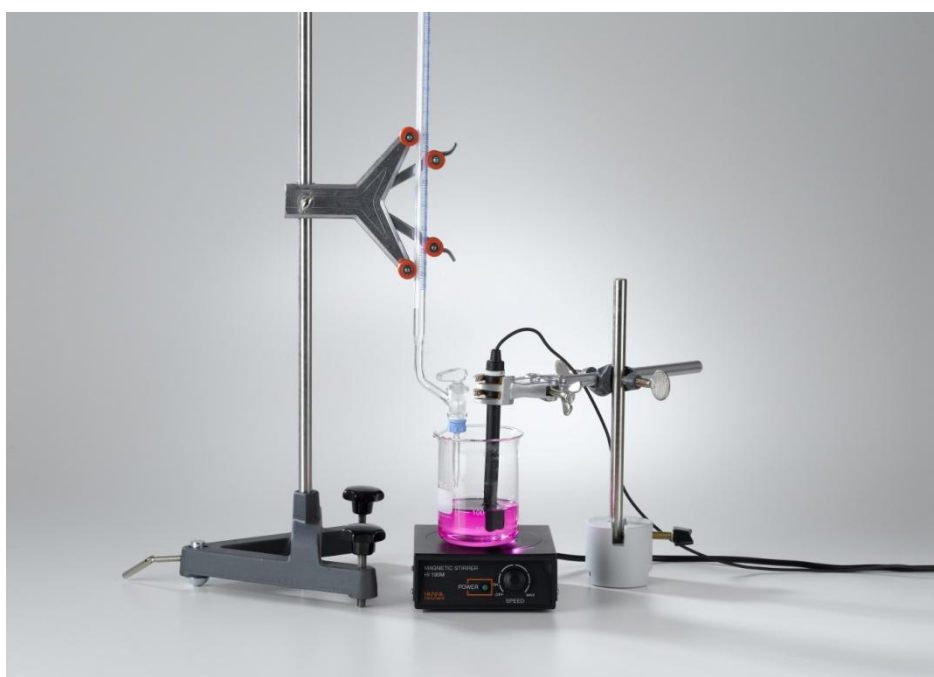
Fig. 1: Experimental set-up for the determination of the acid strength of acetic acid.
