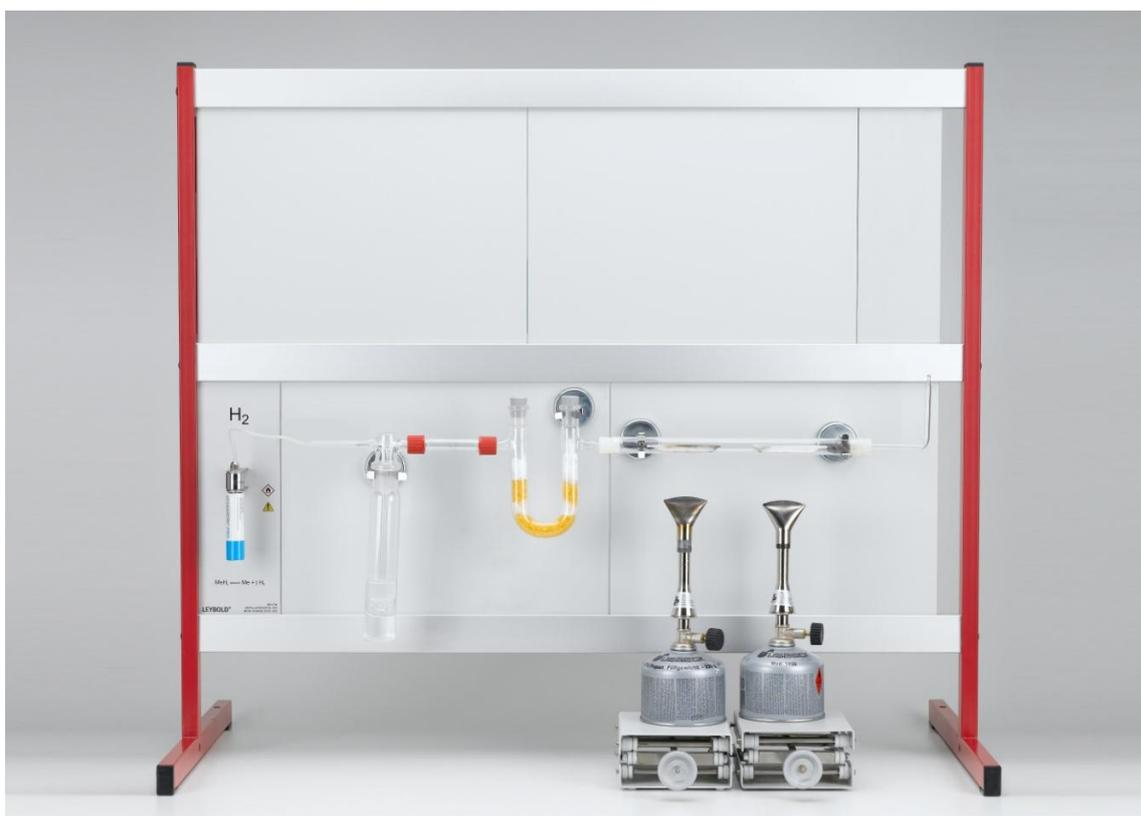
multiple proportions. For this purpose, two different copper oxides are reduced with hydrogen. The different mass ratios in the copper oxides can be experimentally determined by this quantitative reduction. The chemical equations of the redox reactions are as follows:
