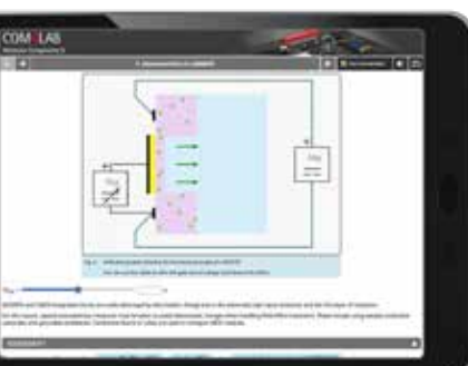
ME1.3.2 - 5. Characteristics of a MOSFET
