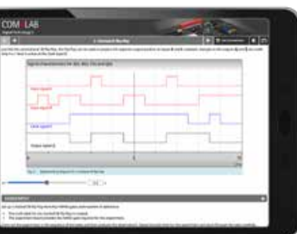
ME1.4.2 - 3. Clocked RS flip-flop
