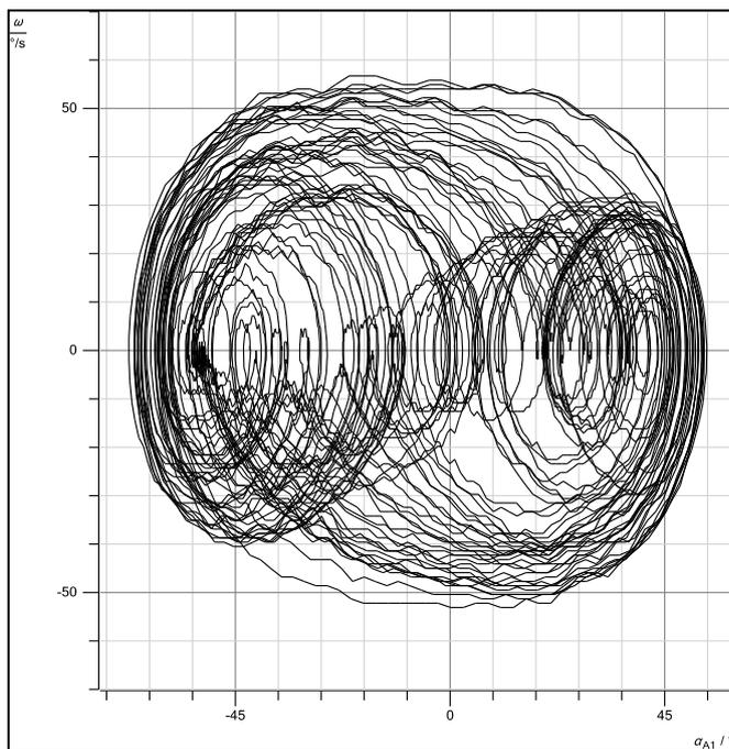
Fig. 11: Phase diagram of the chaotic oscillation. There are no visible closed trajectories.
