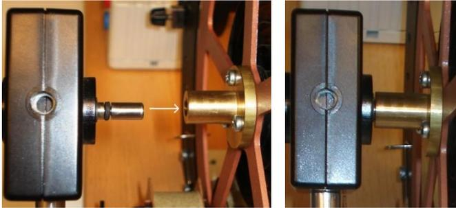
Fig. 3: Mounting of the rotary motion sensor S onto the torsion pendulum.
