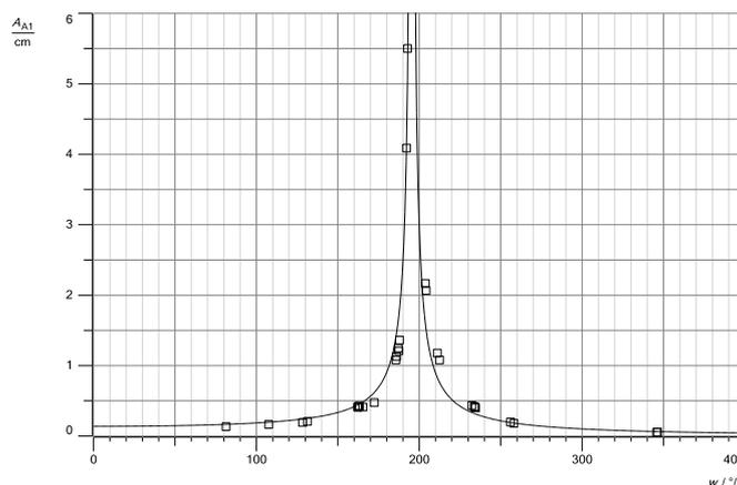
Fig. 8: Resonance curve of the undamped forced harmonic oscillations (different scaling of the axes: for direct comparison with the damped oscillation in the Fig. 7 graph above)
