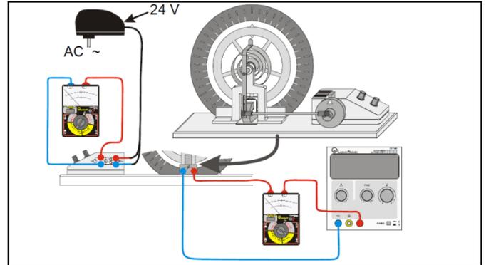
Fig. 5: Connection of the measuring instruments and power supplies.
