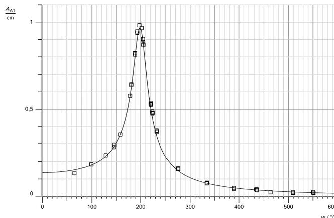
Fig. 7: Resonance curve of the damped forced harmonic oscillations.
