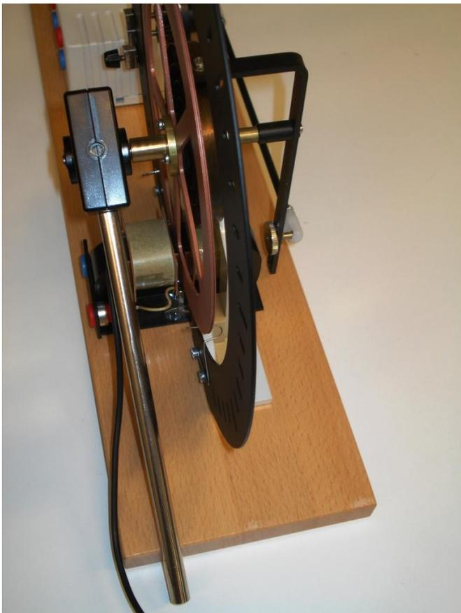
Fig. 4: The rotary motion sensor S on the torsion pendulum.
