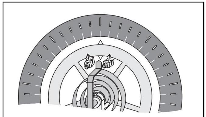
Fig. 6: Mounting of the additional weights to study chaotic oscillations.
