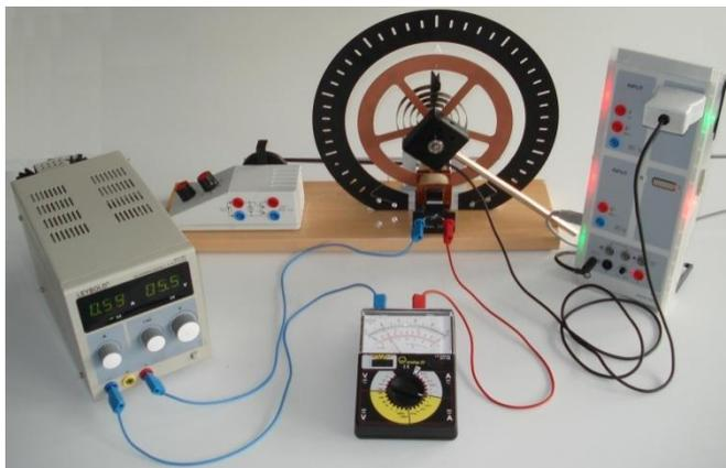
Fig. 1: Experiment setup for forced rotational oscillations.
