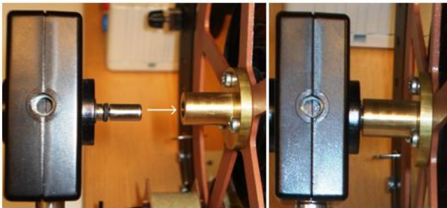
Fig. 2: Mounting of the rotary motion sensor S onto the torsion pendulum
